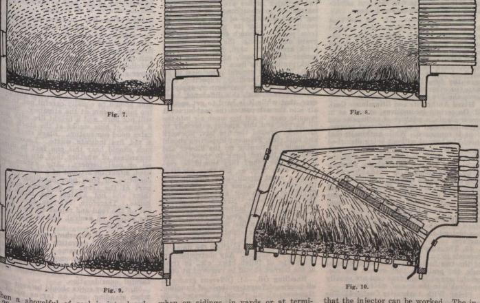
when a shovelful of coal is introduced. 29. Fig. 8 shows the restoration of temperature before the second shovelful is introduced before the most of the fire remperature before the second shovene. is introduced at another part of the fire box, as is the case in the system of light and level cross-firing. 30. Fig. 9 shows the effect of a spot in hole in the firm. The admission of a
