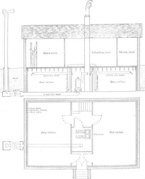
ELEVATION AND GROUND PLAN OF THE CELLAR.
