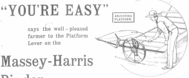
No tugging at chains—a boy can turn the crank to raise or lower Platform.
