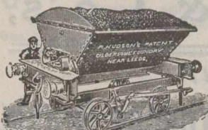
59—R. H.'s Patent 6-Ton Steel Double Side Tip Wagon, to work with ordinary Rly Wagons
