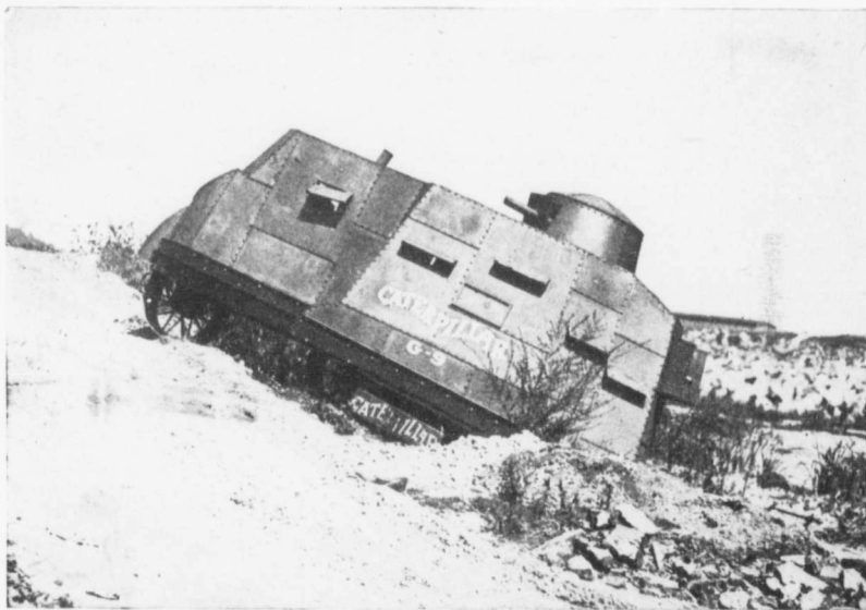
Caterpillar "Tank" Demonstrated to Officers of Army Meets Disaster. A model "Tank" constructed to be demonstrated to officers of the United States Army turned a double somersault while climbing a bank after crossing the Los Angeles River, when the soft earth gave way under the 13-ton machine. The demonstration, however, was successful, as it showed how easily a machine used in time of war can cross a river and climb its banks. The "Tank" is modeled after those in actual service in Europe.
