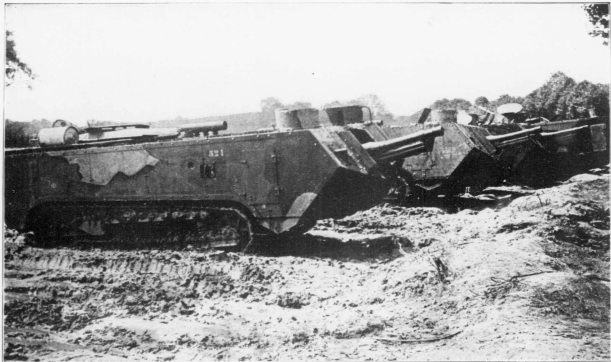
A battery of French St. Chamond tanks in charge formation. The most gigantic and most powerful machines of their type. The long range guns mounted in front are kept working during an advance. They move on the caterpillar chain drive. One of these tanks will house from ten to twenty men.
