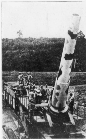
Camouflaged Big Gun. Mounted on a specially constructed railroad carriage, this big French 400 m/m gun was ready to bang away at the German forces making the drive on the Somme front. It was exceedingly well camouflaged to prevent detection by Boche aerial observers.
