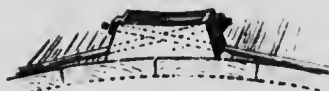
FIG. 8.—Showing clip made of wood or iron to be used where posts are not left in sides.
