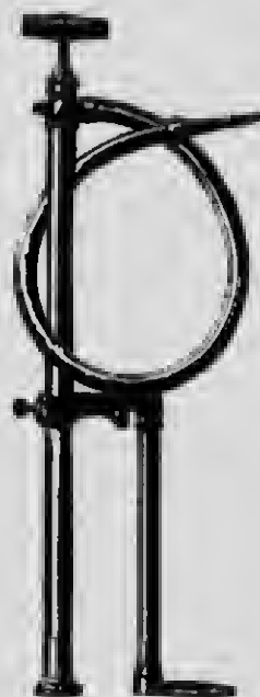
FIG. 246.—Bucket force pump.
