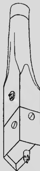
FIG. 253.—Tool for cutting cards of tarred building paper. (After Slingerland.)
