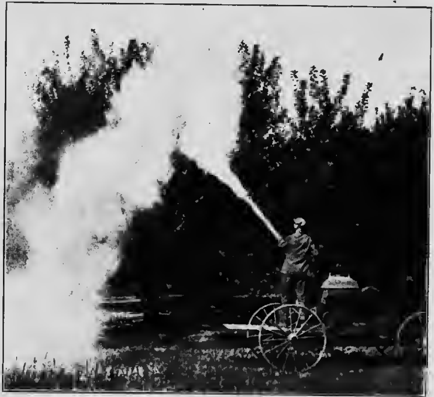
FIG. 249.—A dust sprayer in operation in an orchard. (Courtesy of the Niagara Sprayer Co.)
