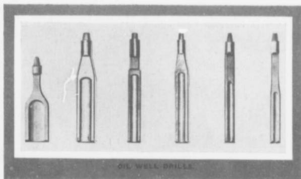
The standard or cable drilling system is used in hard rock, and the rotary in softer formation, while frequently both are combined.
