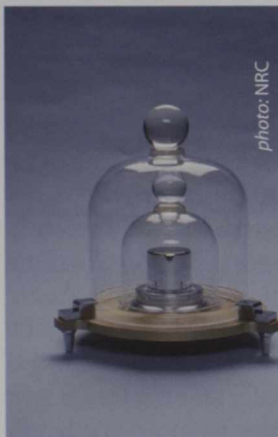
Canada's reference kilogram weight under two glass jars at the NRC.
