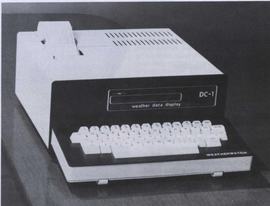
Weatherwatch digital readout and processor unit
