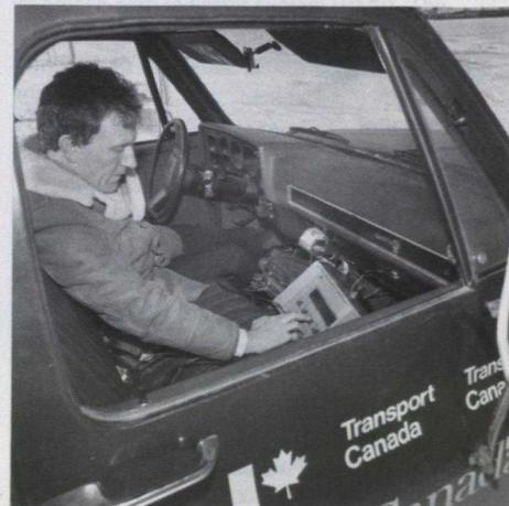
Operator using portable signal analyzer
