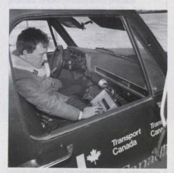
Operator using portable signal analyzer
