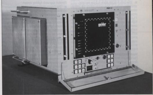
GUIDAR processor/display unit
