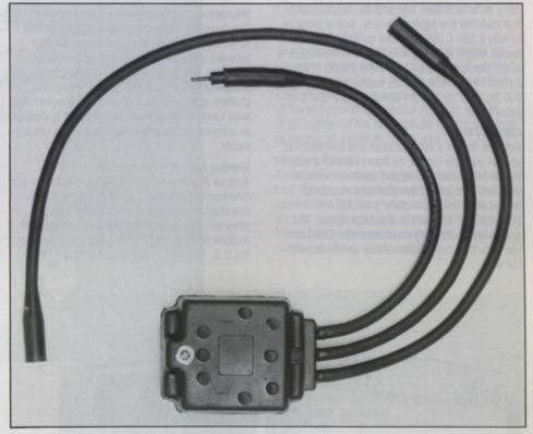
Polychloroprene encapsulated isolating transformer with earthing stud
