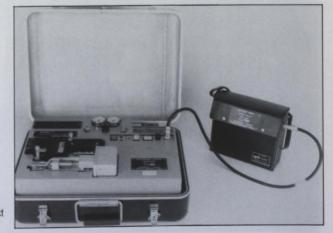
The Scintrex EVD-1, designed to detect vapours from concealed explosives
