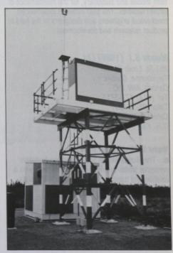
MLS azimuth transmitter
