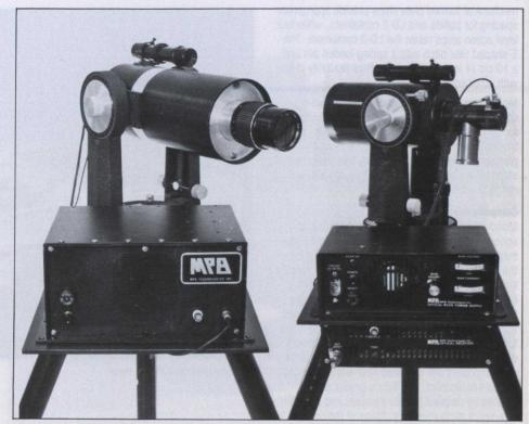
Laser communication receiver and transmitter
