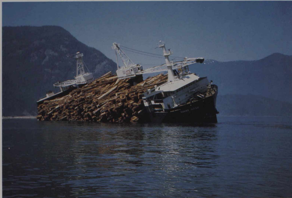
This self-dumping log carrier moves timber from the remote Queen Charlotte Islands down the B.C. coast to the mills, where it unloads by taking on water and tilting to a 30-degree angle.
