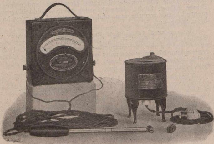
Fig. 1.—Recalcescent Outfit. Note the two test specimens of steel, one fastened to couple.
