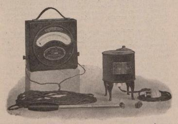
Fig. 1.-Recalescent Outfit. Note the two test specimens of steel, one fastened to couple.
