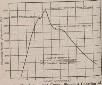
Fig. 2.-Heating-cooling Curve, Showing Location of "Critical Temperatures."
