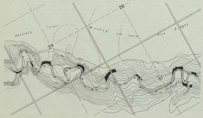
Example of topographic maps recently completed by S. C. Ells, illustrating typical mode of occurrence of bituminous sand deposits in Northern Alberta. All streams tributary to the Athabaska riverin the McMurray district have been mapped in this manner. The maps were originally drawn on a scale of 1 inch equals 400 feet, but have been reduced to the present scale of 1 inch equals 1000 feet.
