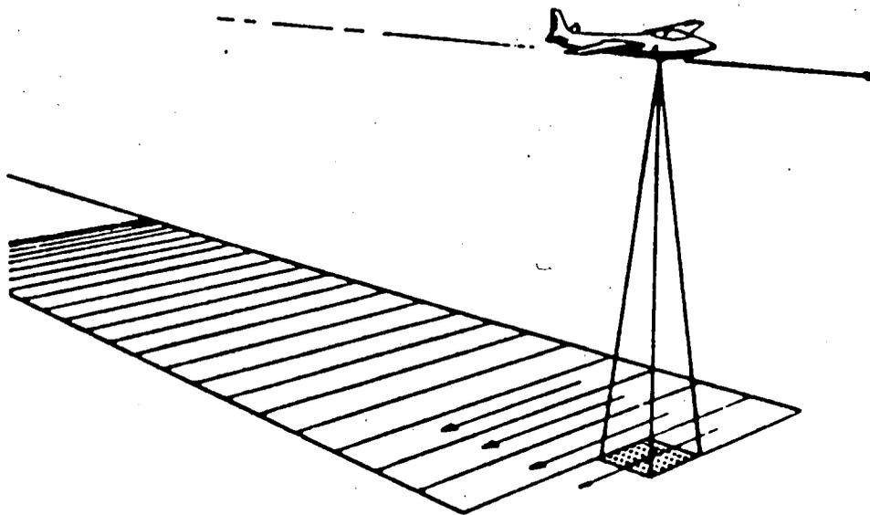
Figure 14. Operation of an airborne line scanner to produce contiguous imagery. Rotation of the mirror provides the across-track dimension of the image. The forward motion of the aircraft causes successive scan lines to cover adjacent strips on the ground, forming the second dimension of the image. (Source: Madding, Robert P. 1979. Thermographic instruments and systems. University of Wisconsin-Extension. Department of Engineering and Applied Science. p. 82.)
