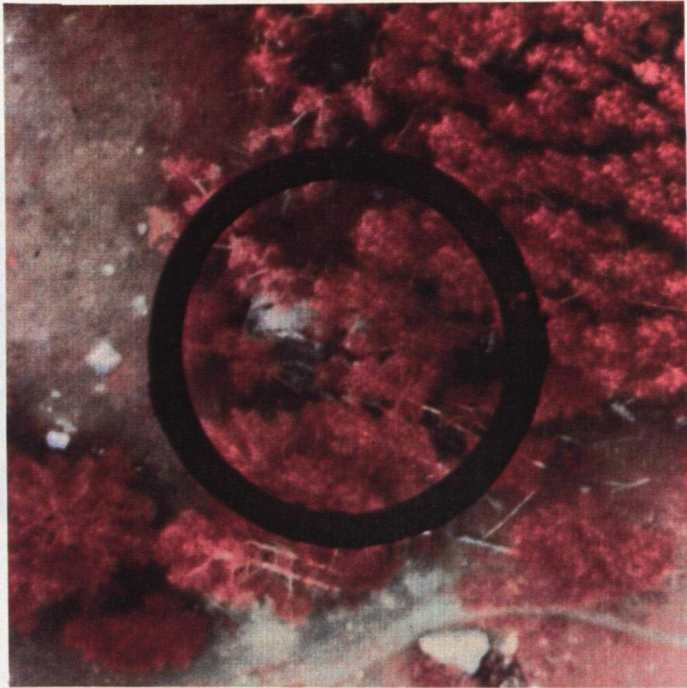
Figure 11. Colour infrared film can be useful to detect poorly camouflaged military equipment. The camouflage net in this photograph does not match the spectral characteristics of the surrounding vegetation, making it visible in the photo. (Courtesy of David Dorschner, Aerial Intelligence Specialists)
