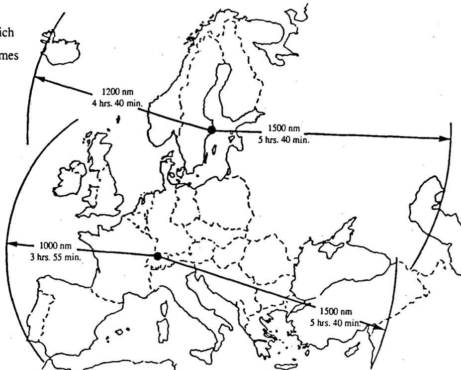
Figure 22. Typical ferry distances and times for Dash 8 Series 300 aircraft based out of Stockholm and Zurich. (Source: Airborne Remote Sensing for C.F.E. Verification: The Platform. op. cit., p. 15.)
