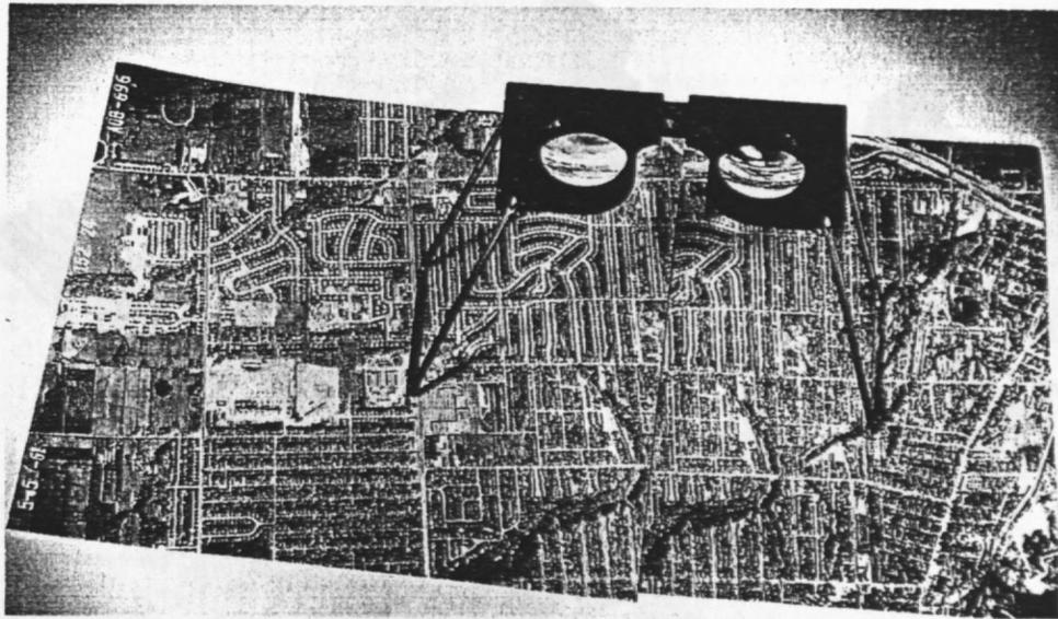
Figure 4. A simple "pocket" stereoscope. (Source: Lillesand and Kiefer, op. cit., p. 103.) transparency roll film. (Source: Colwell, Robert N. (editor-in-chief). 1983. *Manual of Remote Sensing*. 2nd Edition. Volume 1: Theory, Instruments and Techniques. American Society of Photogrammetry. Falls Church, VA. p. 101b.)
