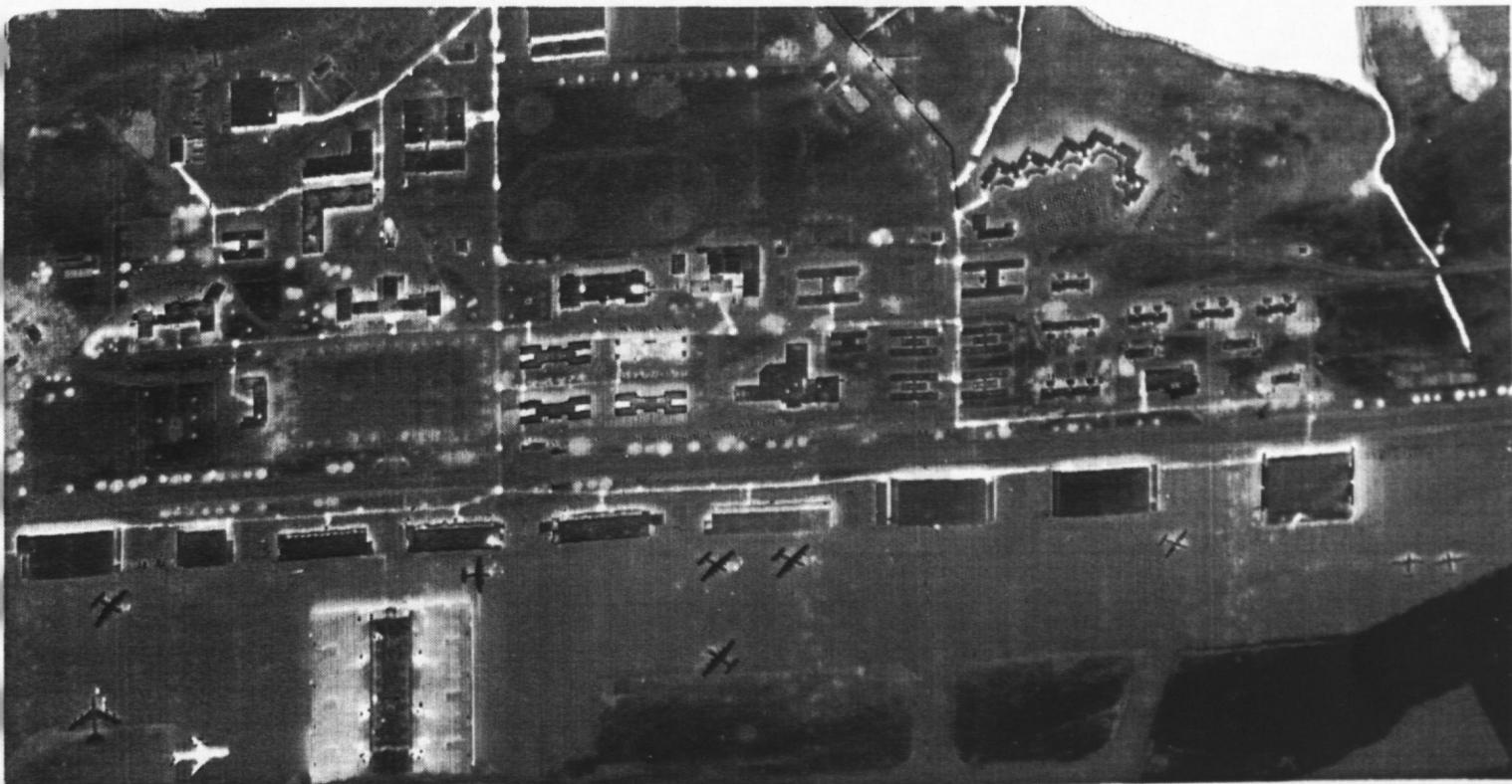
Figure 15. Thermal infrared linescan image of an airport. White is "hot" and black is "cold" in this image. The image was taken at night. Notice the "hot" buried steamlines and trees along the roadsides. Warm auxillary power units (APU's) can be seen near some of the aircraft. One aircraft appears anomalously warm compared to the others. It may have been parked inside the nearby hangar not long before the image was acquired. (Courtesy of Intera Technologies Ltd.)
