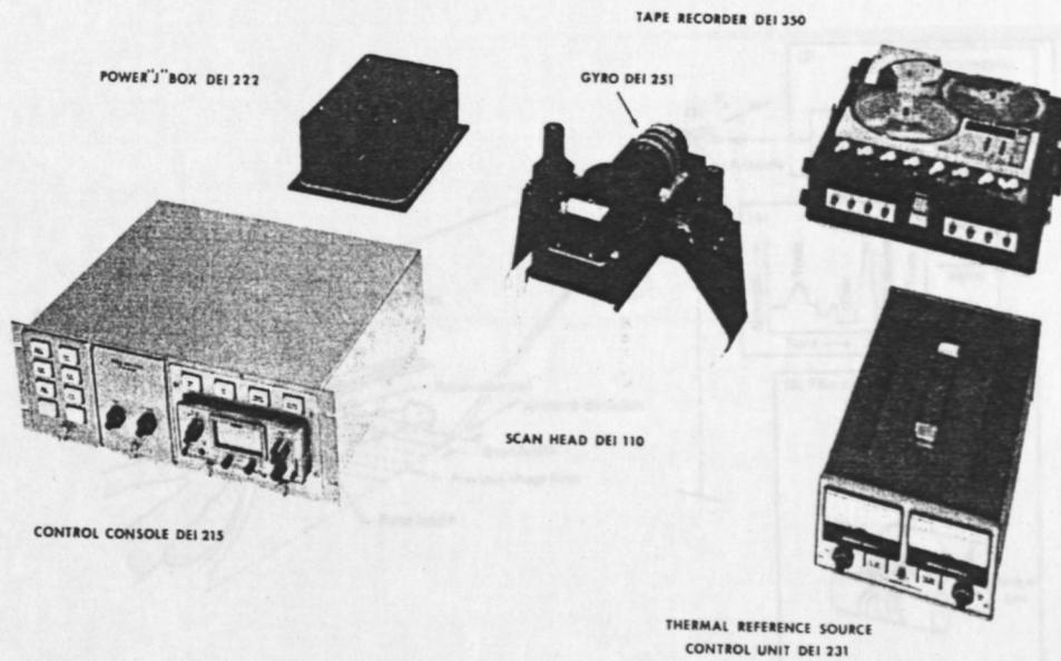
Figure 16. Thermal infrared linescanner system including the scan head, control console, blackbody reference source control unit, tape recorder and "J" box. (Source: Lillesand and Kiefer, op. cit., p. 402.)
