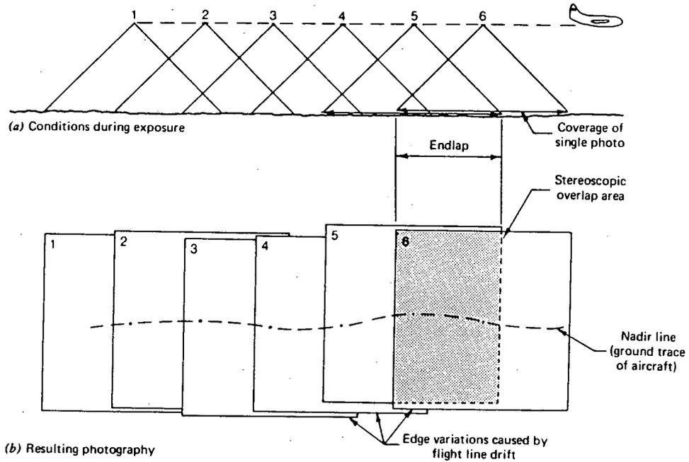
Figure 2. Acquisition of overlapping photographic coverage along a flight strip to provide stereoscopic coverage. (Source: Lillesand, Thomas M. and Ralph W. Kiefer. Remote Sensing and Image Interpretation. John Wiley & Sons. New York. p. 78.)
