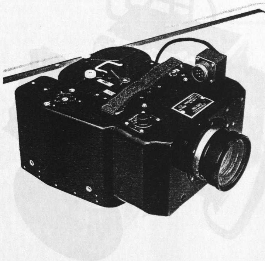
Figure 8. The Vinten Type 1360 reconnaissance camera complete with automatic exposure control and 6 inch lens. The film magazine holds 500 exposures on 70 mm film. (Source: Graham, Ron and Roger E. Read. 1986. Manual of Aerial Photography. Focal Press. London. p. 44.)
