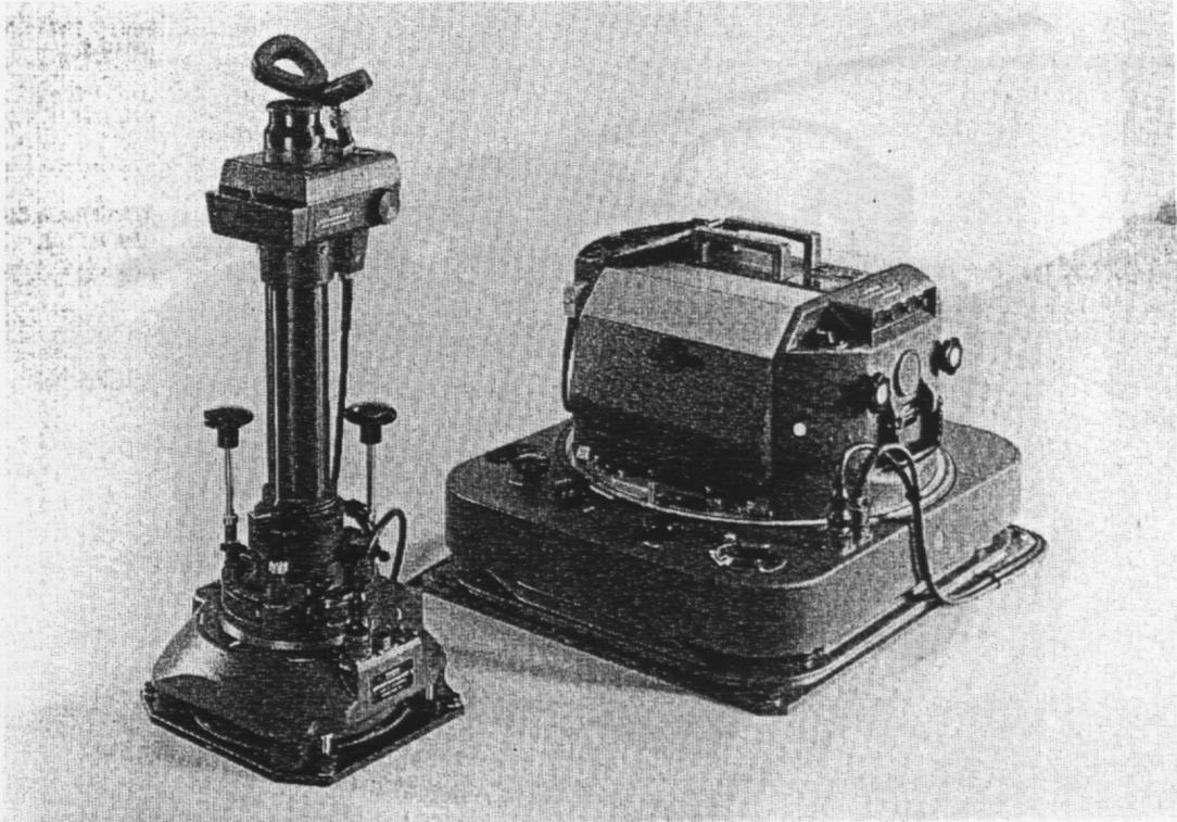
Figure 7. The Wild AVIOPHOT RC20 Aerial Camera System with camera (right) and navigation sight (left). (Courtesy of Wild Heerbrugg Ltd.)
