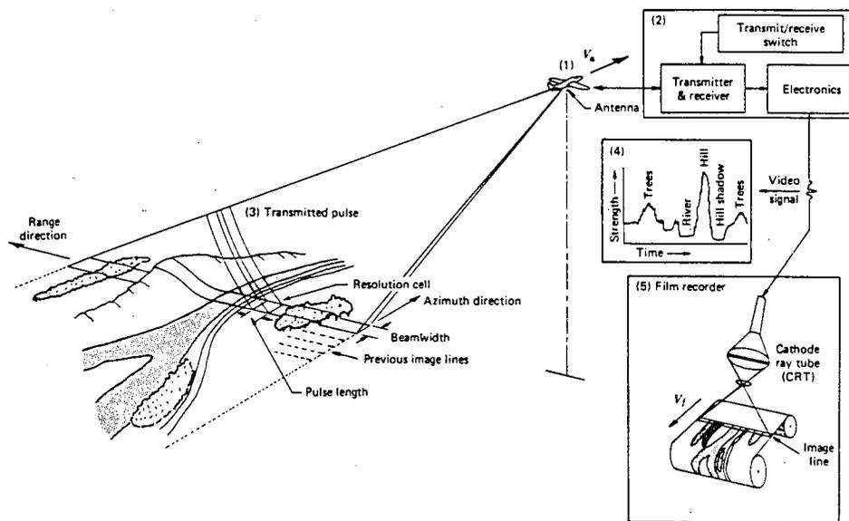
Figure 17. Operation of a real aperture side-looking airborne radar (SLAR). (Source: Lillesand and Kiefer, op. cit., p. 495.)
