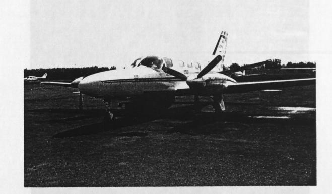
Figure 20. Twin-engined Cessna Conquest equipped with synthetic aperture radar. The Conquest is a costeffective platform which delivers the altitude, range and speed capabilities required to operate a SAR. The aircraft would also make a good platform for an infrared linescanner or mapping camera. (Courtesy Intera Technologies Ltd.)
