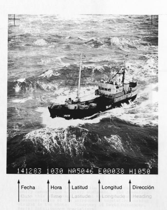
Figure 10. Oblique photograph taken using an Agiflite hand-held camera with time and position data in the margin, recorded at the time of exposure. (Courtesy of Negretti Aviation)
