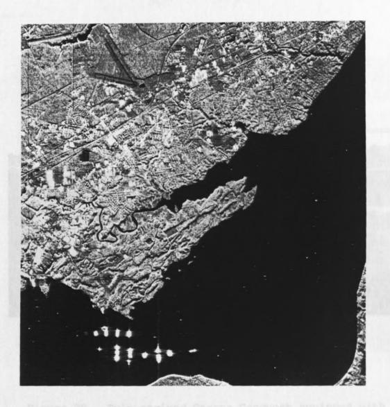
Figure 19. The tethered destroyers seen as bright returns near the bottom of this SAR image are plainly visible but not necessarily easy to identify. Many common cultural features, such as roads, an airport, and housing subdivisions, are evident. (Courtesy of Intera Technologies Ltd.)
