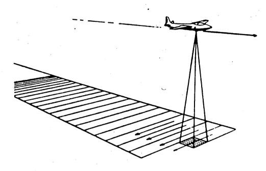
Figure 14. Operation of an airborne line scanner to produce contiguous imagery. Rotation of the mirror provides the across-track dimension of the image. The forward motion of the aircraft causes successive scan lines to cover adjacent strips on the ground, forming the second dimension of the image. (Source: Madding, Robert P. 1979. Thermographic instruments and systems. University of Wisconsin-Extension. Department of Engineering and Applied Science. p. 82.)
