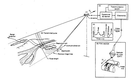
Figure 17. Operation of a real aperture side-looking airborne radar (SLAR). (Source: Lillesand and Kiefer, op. cit., p. 495.)
