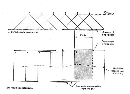
Figure 2. Acquisition of overlapping photographic coverage along a flight strip to provide stereoscopic coverage. (Source: Lillesand, Thomas M. and Ralph W. Kiefer. <u>Remote Sensing and Image Interpretation</u>. John Wiley & Sons. New York. p. 78.)
