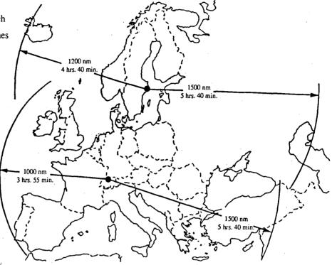
Figure 22. Typical ferry distances and times for Dash 8 Series 300 aircraft based out of Stockholm and Zurich. (Source: <u>Airborne Remote Sensing for C.F.E.</u> <u>Verification: The Platform</u>. op. cit., p. 15.)
