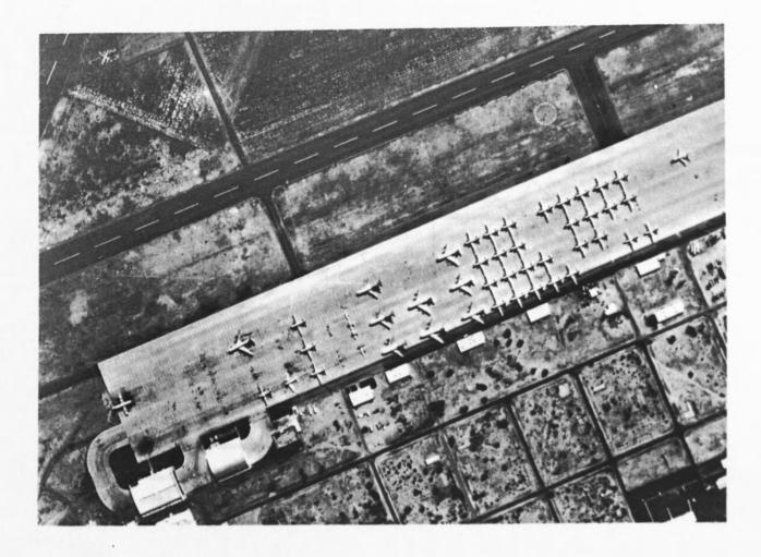
Figure 1. Typical vertical panchromatic aerial photograph of an airfield. Several different kinds of aircraft can be distinguished. (Courtesy of Intera Technologies Ltd.)
