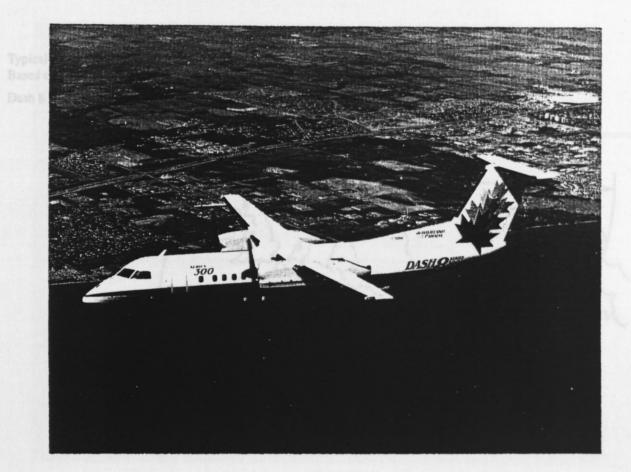
Figure 21. The de Havilland Dash 8 Series 300 provides a platform with room for 16 passengers or more as well as a full complement of sensors. Based from a central location in Europe, the Dash 8 could reach any target within the "Atlantic to the Urals" region within six hours without refueling. The Dash 8's airfield performance would permit operations from most airfields in Europe. (Courtesy of Boeing Canada, de Havilland Division)
