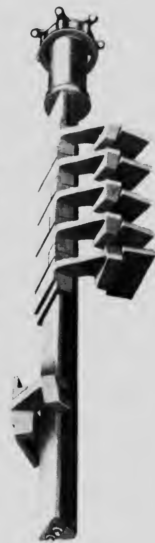
1. Rabble arm 2. Arm dressed with rabble blade holders and blades 3. Arm partly dressed with holders and breech block
