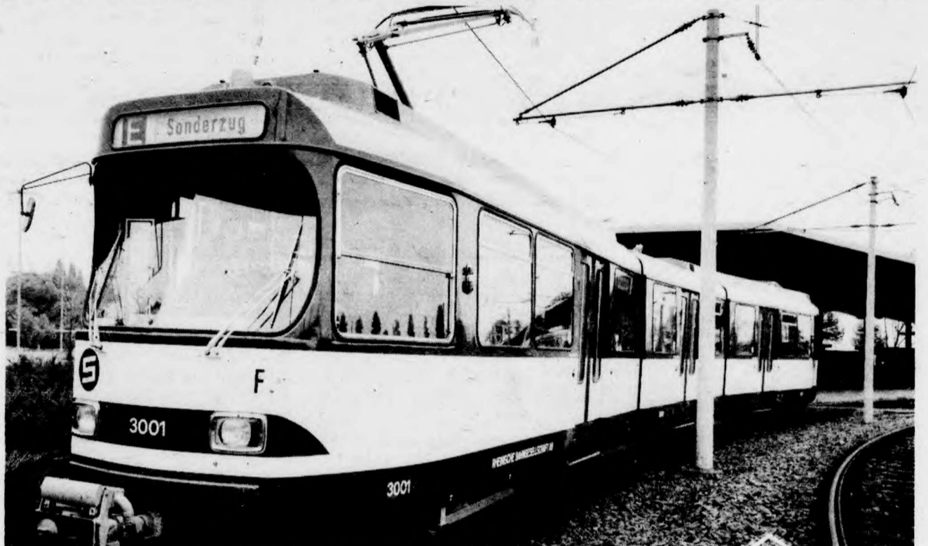
New streetcars on Spadina Ave. may be more than just streetcars, namely Light Rapid Transit (LRT) vehicles. A typical example of new generation LRT used across Europe is this 3-section (for bending
