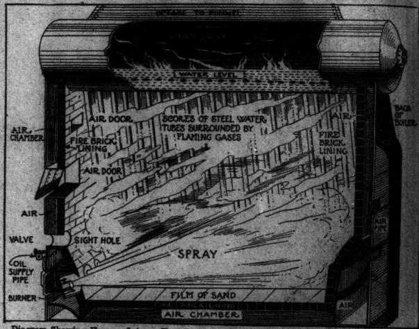
Diagram Showing How an Intense Heat Is Generated by the Use of Oil as Fuel.
