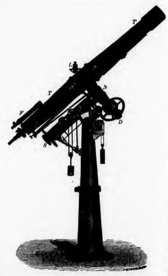
FIG. 37.—EQUATORIAL TELESCOPE POINTED TOWARD THE POLE.
