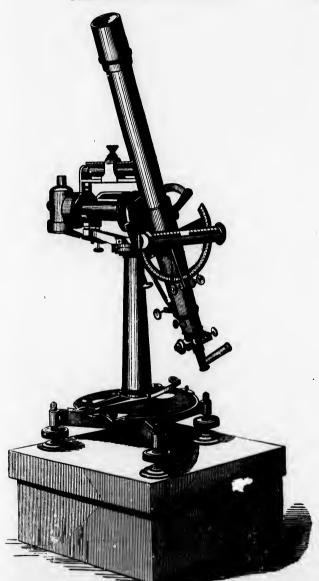
Fig. 39.—THE ZENITH TELESCOPE.
