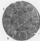
Locked Coil Aerial Cable or Colliery Guide.
