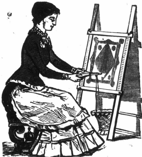
The above cut illustrates a Novelty Rug Machine, which is employed for making rugs, tidies, door mats, mittens, hoods, etc. It is very simple in construction, and is worked with ease and rapidity.
