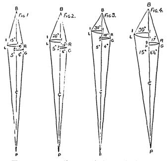
The proportions in Fig. 2 give both a good safety and impulse action and can be used for ordinary as well as fine work.
