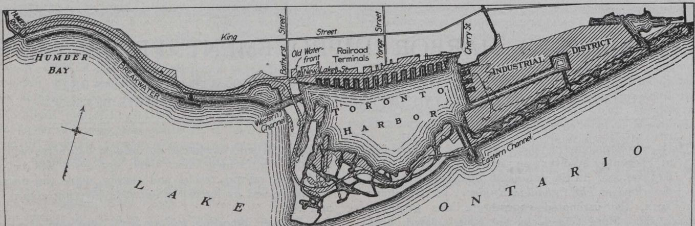
Fig. 2.—General Plan of Improvements Under Way. Hatched Portion Indicates Reclaimed Areas.
