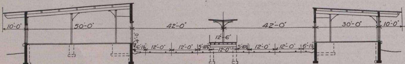
Fig. 2.—Section (G-H) Through Freight Sheds and Transfer Platforms.
