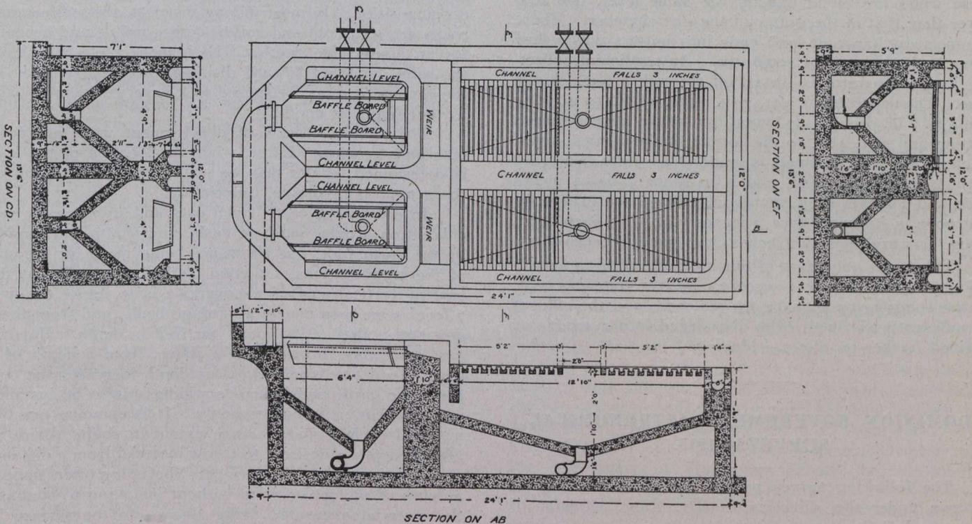
Plan and Sections of Chilliwack Separator
