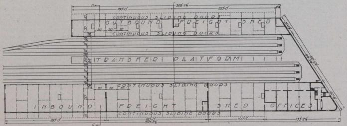
Fig. 1.-Layout of C.P.R. Freight Terminals at Quebec.
