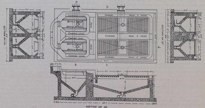
Plan and Sections of Chilliwack Separator
