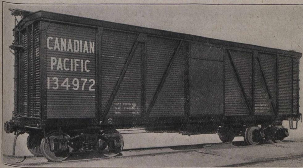
Standard Canadian Pacific Railway Steel Frame Car Fitted with Corrugated Steel Lining.
