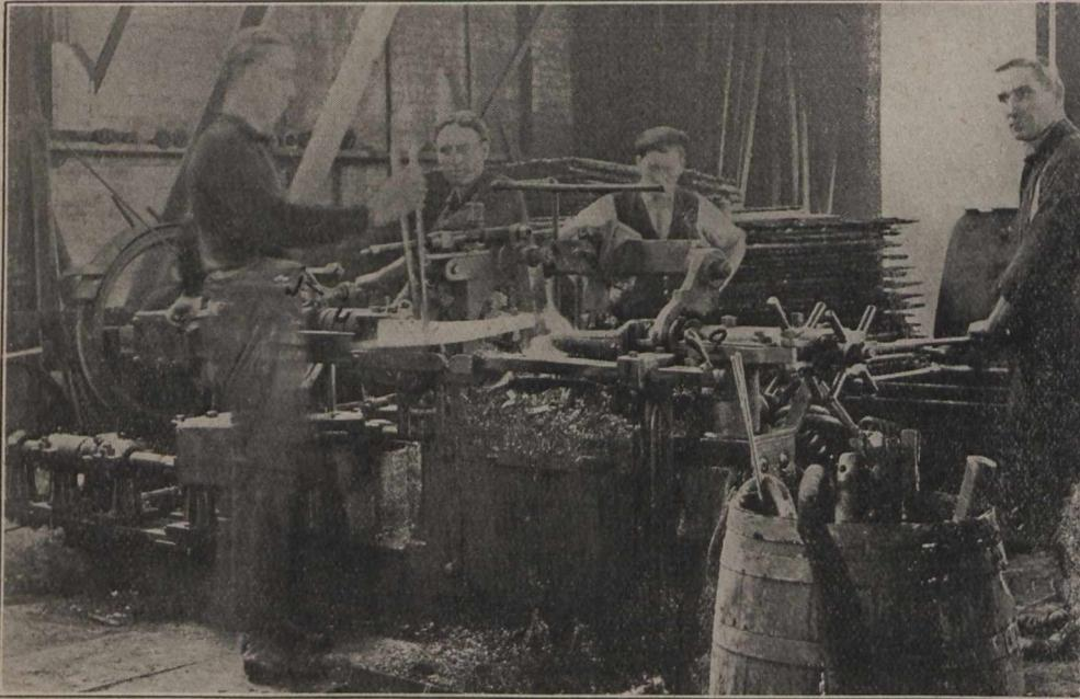
Fig. 1.—Coil Winding Machine.
