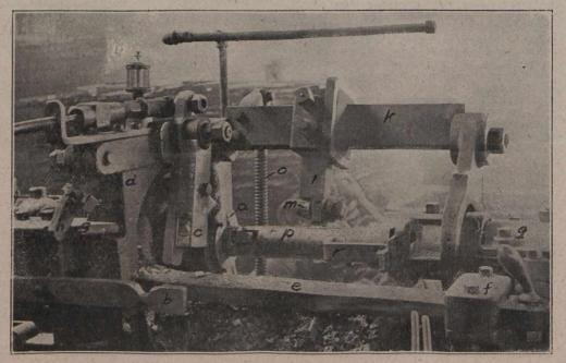
Fig. 2 .--- Close View of Coil Machine.
