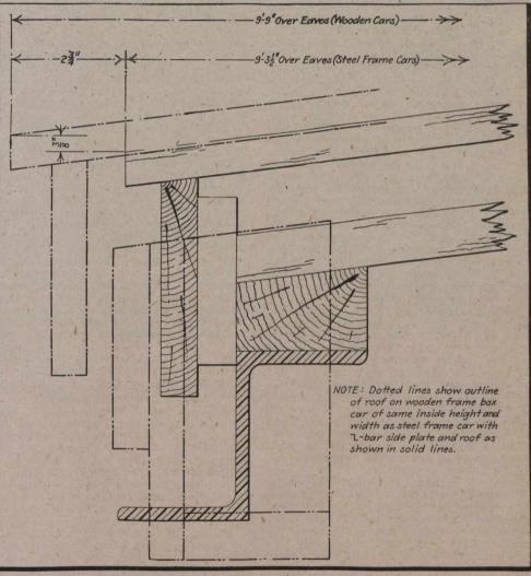
Details of Roof Clearances on Steel and Wooden Box Cars.
