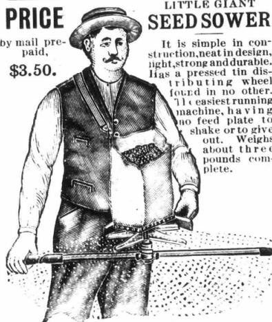
It is simple in construction, neat in design, light, strong and durable. Has a pressed tin distributing wheel found in no other. The easiest running machine, having no feed plate to shake or to give out. Weighs about three pounds complete.
