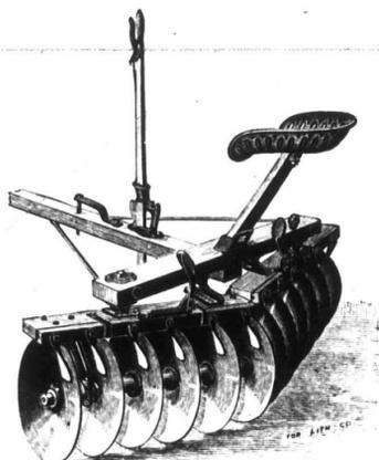
Pronounced by the Farmers to be perfection. All Steel Discs, with the latest improved Scrapers. Don't fail to see our 1891 scrapers; the point we claim on these is, they are not constantly rubbing on the Disc, causing friction, and thereby adding to the draft. To clean Discs, simply touch foot to spring on side of seat, this brings Scrapers in contact with Discs, cleaning them instantly. Our new Hinges are so constructed as to allow the flexibility desired.
