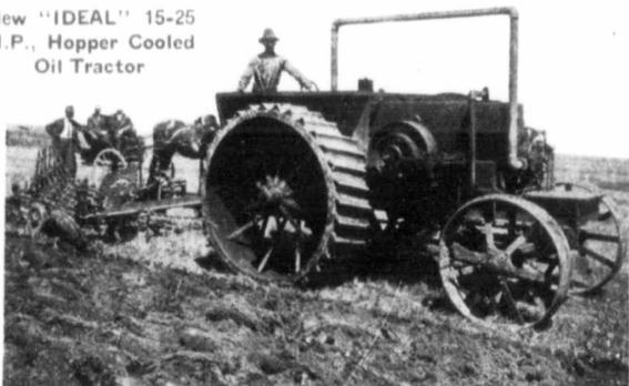
For your next spring's work you should investigate the New "Ideal" Light Weight 15-25 H.P. Opposed Cylinder, Hopper Cooled Oil Tractor. This tractor was built for field experience and is built right. We also, build Oil Tractors of 18-35 and 25-50 H.P.
