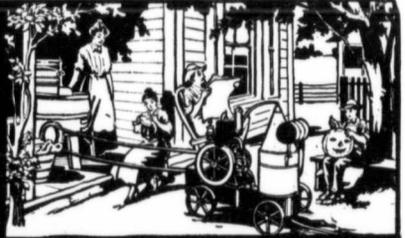
8 h.p. 2-Cylinder Cushman mounted on hay press. Engine weighs only 320 lbs. This engine may be mounted on iron truck and pulled around by hand.
