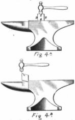
under the flatter; in this case, it is held on the anvil lengthwise and the flatter held against the upper face parallel to the face of the anvil, while the helper strikes a few light blows.
