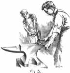
be held as shown in Fig. 2b. The drawing may be done by holding the work across the horn of the anvil, the sharper curve causes the metal to flow more freely than on the face, but it is more liable to cause irregularities in the shape. When the work is to be straightened, it should be laid lengthwise, as shown in Fig. 2b, because the anvil is straight in this direction
