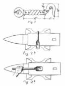
by means of specially formed dies between which or into which the metal is pressed or hammered. Welding is the process of uniting two pieces of metal into one solid piece by heating them to a welding heat and hammering or pressing them together. For wrought iron, a white heat is necessary to soften the metal so that it will weld.
