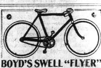
1900 MODEL. New ideas, new design, 13/in. tubing, flush joints, Springfield one-piece cranks, high grade in every detail. Fitted with Victor tires, \$35.00; with Morgan & Wright tires, \$37.50; with Dunlop tires, \$40.00. Men's, 22 and 24 inch; Ladies', 20 and 22 inch frames. Black and maroon
