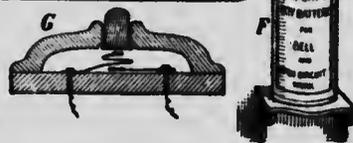
through the electromagnet to the battery. The armature is drawn in and the bell struck by the hammer; but by the
