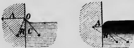
FIG. 184.—Diagrams to explain capillary action.
