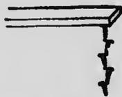
FIG. 448.—A chain of magnets by induction.
