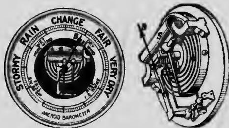
FIG. 134. — Aneroid barometer.
