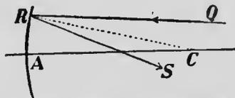
FIG. 313.—Reflection from a concave mirror.
