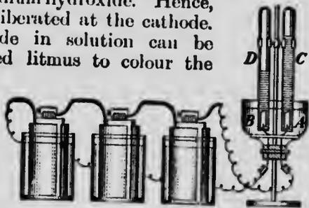
FIG. 406.—Electrolysis of water.
