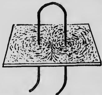
FIG. 516.—Magnetic field of currents in opposite directions.
