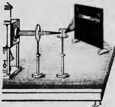
FIG. 402.—Showing how to produce a pure spectrum.
