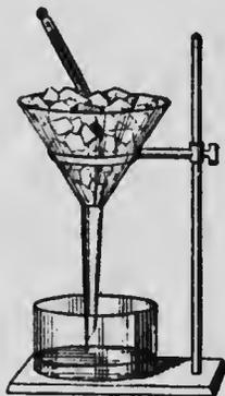
FIG. 265. — Determination of freezing point.
