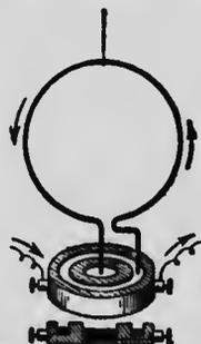
FIG. 505.—Experiment to show that a circular loop carrying a current behaves as a disc magnet.
