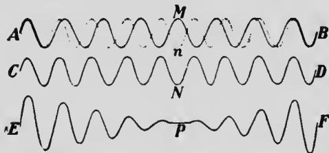
FIG. 239.—Illustrating the production of beats. The combination of *AB* with *CD* gives *EF*. The dotted curve in *AB* is the same as the curve *CD*. At *M* the motion is up, at *N* it is down, and these added give us motion as at *P*.
