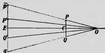
FIG. 432.—The magnification is the ratio of  $p'q'$  to  $PQ$ .
