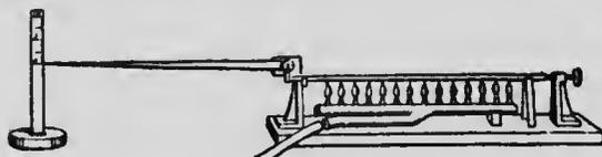
FIG. 255.—Expansion of rod by heat.
