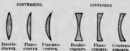
FIG. 380.—Lenses of different types.
