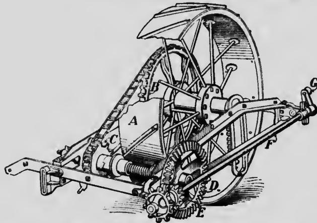
driving-wheel *A* has a diameter of 3 feet, the sprocket-wheels *B* and *C* have 40 teeth and 10 teeth, respectively. The large gear-wheel *D* has 37 teeth and the small one *E* has 12 teeth, and the crank *G* is 3 in. long. Neglecting friction, what pull on the driving-wheel
