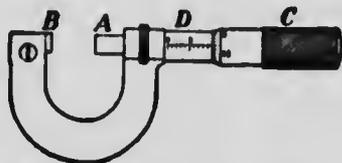
FIG. 7.—Micrometer wire gauge.
