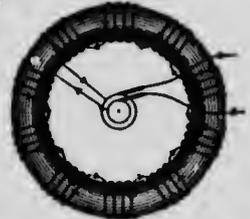
FIG. 535.—Gramme-ring armature. (Invented by Gramme in 1868.)
