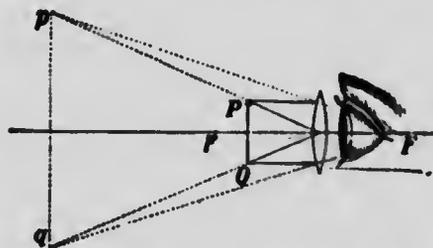
FIG. 431.—Illustrating the action of the simple microscope.
