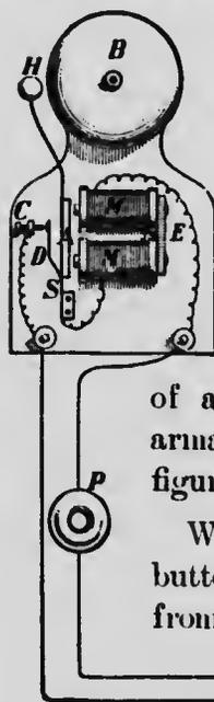
FIG. 521.—Electric bell and its connections. At *G* is shown a section of the push-button. The figure shows the bell when the button is not pressed. The current may pass in either direction through the bell.
