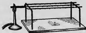
FIG. 301.—Difference in conductivity of metals.
