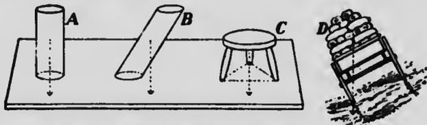
FIG. 57.—*A* and *C* are in stable equilibrium; *B* is not, it will topple over; *D* is in the critical position.
