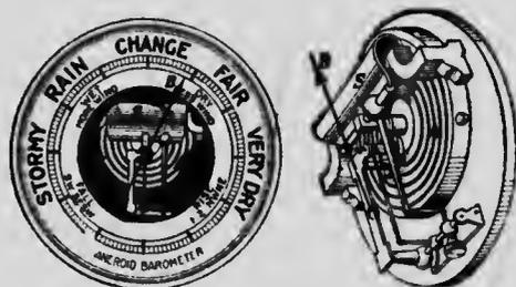
FIG. 134. — Aneroid barometer.
