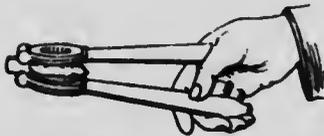
FIG. 71.—Nut-crackers, lever of the second class.
