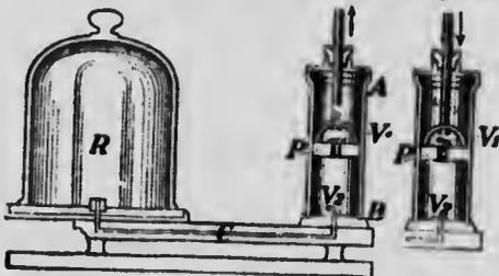
FIG. 147.—Common form of air-pump.  $AB$ , cylindrical barrel of pump;  $R$ , receiver from which air is to be exhausted;  $C$ , pipe connecting barrel with receiver;  $P$ , piston of pump;  $V_1$  and  $V_2$ , valves opening upwards.
