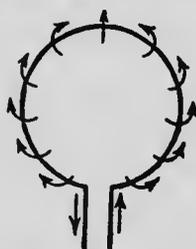
FIG. 504.—Lines of force about a circular loop.
