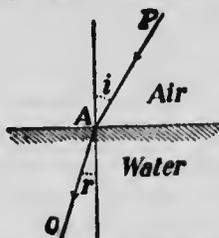
FIG. 362.—Illustrating refraction from air to water.
