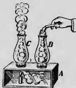
FIG. 310.—Convection currents in heated air.
