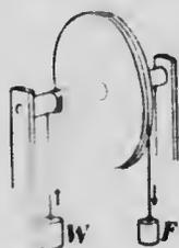
FIG. 87.—The wheel and axle.
