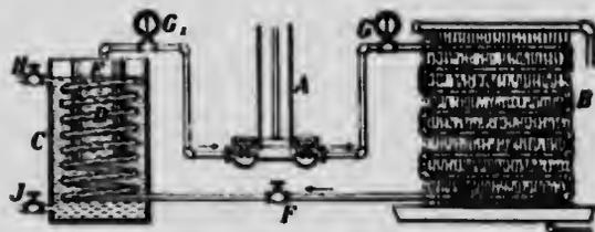
FIG. 286.—Ice-making machine. *G*<sub>1</sub>, high-pressure gauge; *G*<sub>2</sub>, low-pressure gauge; *A*, pump for exhausting low-pressure coils and condensing gas; *B*, condenser coils cooled by running water from a pipe placed above them; *F*, regulating valve; *D*, low pressure coils; *C*, tank containing brine; *E*, can containing water to be frozen.
