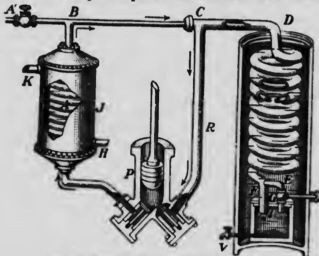
FIG. 288.—Essential parts of a liquid-air machine.
