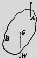
FIG. 53.—How to find the centre of gravity of a body of any form.
