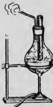
FIG. 275.—Determination of specific heat of a solid.
