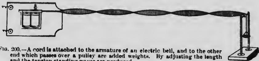
FIG. 200.—A cord is attached to the armature of an electric bell, and to the other end which passes over a pulley are added weights. By adjusting the length and the tension standing waves are produced.
