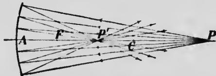
FIG. 351.—Conjugate foci in a concave mirror.  $P$  and  $P'$  are conjugate.
