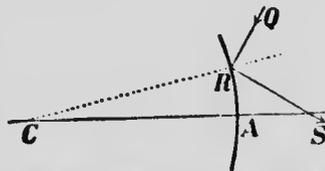
FIG. 314.—Reflection from a convex mirror.
