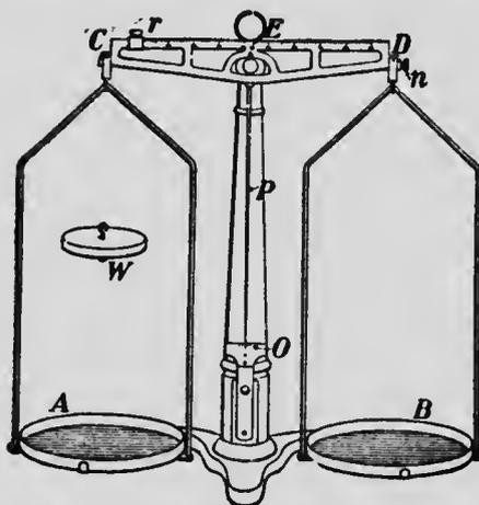
FIG. 8—A simple and convenient balance. When in equilibrium the pointer *P* stands at zero on the scale *O*. The nut *n* is for adjusting the balance and the small weights, fractions of a gram, are obtained by sliding the rider *r* along the beam which is graduated. The weight *W*, if substituted for the pan *A*, will balance the pan *B*.
