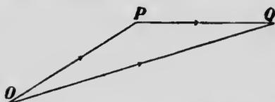
FIG. 12.—The addition of displacements.
