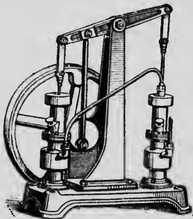
FIG. 148. — An oil air-pump with two cylinders.
