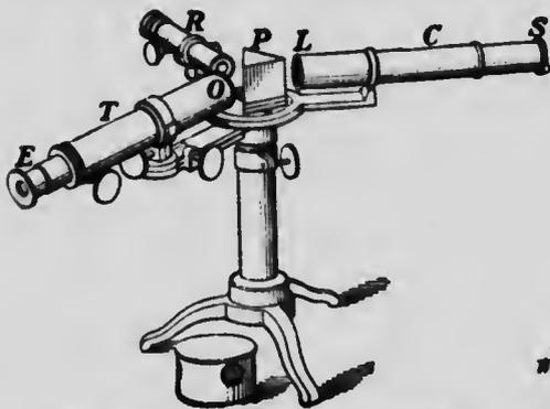
FIG. 417. — A single-prism spectroscope.
