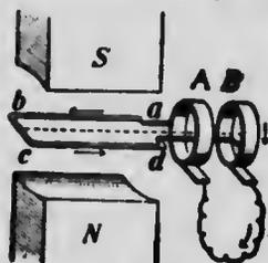
FIG. 530.—Principle of the dynamo.
