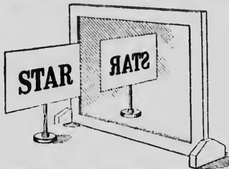
FIG. 338.—Illustrating "lateral inversion" by a plane mirror.
