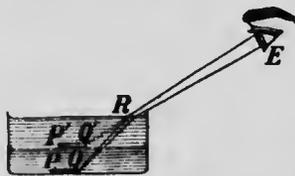
FIG. 363.—The bottom of the vessel appears raised up by refraction.
