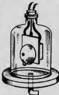
FIG. 201.— Electric bell in a jar connected to an air-pump. On exhausting the air from the jar the sound became weaker.
