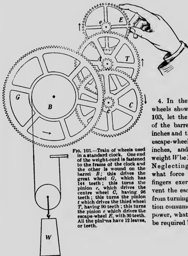
FIG. 103.—Train of wheels used in a standard clock. One end of the weight-cord is fastened to the frame of the clock and the other is wound on the barrel *B*; this drives the great wheel *G*, which has 144 teeth; this turns the pinion *c*, which drives the centre wheel *C*, having 96 teeth; this turns the pinion *t* which drives the third wheel *T*, having 90 teeth; this turns the pinion *e* which drives the escape-wheel *E*, with 30 teeth. All the pinions have 12 leaves, or teeth.
