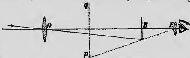
FIG. 435.—The astronomical telescope.
