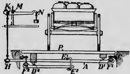
Fig. 102.—Diagram of multiplying levers in a scale for weighing hay, coal and other heavy loads. In the figure is shown one half of the system of levers, as seen from one end. The platform *P* rests on knife-edges *D*<sup>1</sup>, *D*<sup>2</sup>, the former of which is on a long lever, the latter on a short one. The knife-edges *F*<sup>1</sup>, *F*<sup>2</sup> at the ends of these levers are supported by suspension from the brackets *C*, *C* which are rigidly connected with the earth.
