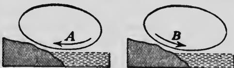
FIG. 311.—Illustration of land and sea breezes. *A*, direction of movement in sea breeze. *B*, direction of movement in land breeze.
