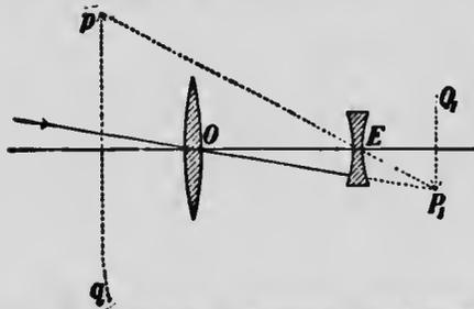
FIG. 438.—A section of the ordinary opera glass.
