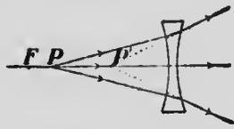
FIG. 390.—Conjugate foci in a diverging lens.
