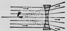
FIG. 382.—In a diverging the principal focus  $F'$  is virtual.
