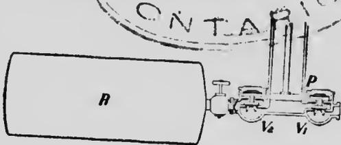
FIG. 153.—Air-compressor. *P*, piston; *R*, tank or receiver; *V*<sub>1</sub> inlet valve; *V*<sub>2</sub> outlet valve.
