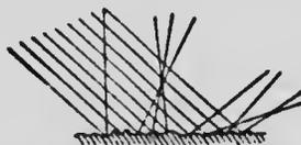
FIG. 336.—Scattering of light from a rough surface.
