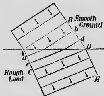
FIG. 365.—Illustrating how a change in direction of motion may be due to change in speed.
