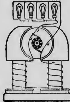
FIG. 545.—Shunt-wound dynamo.
