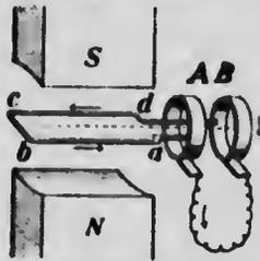
FIG. 532.—Principle of the dynamo.
