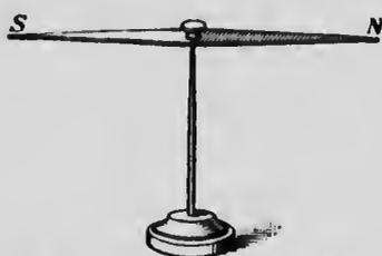
FIG. 444.—A compass-needle magnet.
