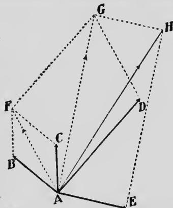
FIG. 25.—How to combine more than two velocities.
