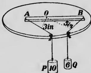
FIG. 37.—Apparatus for testing the law of moments.
