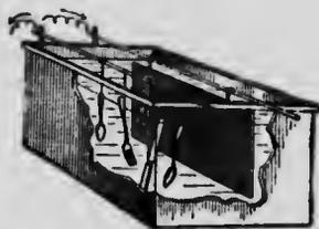
Fig. 497.—Bath and electrical connection for electroplating.
