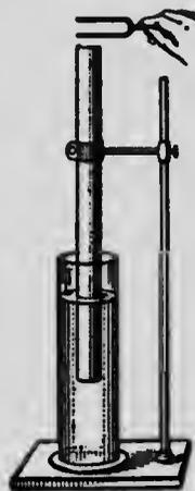
FIG. 222. — Air column in resonance with a tuning-fork.
