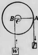
FIG. 88.—Diagram to explain the wheel and axle.
