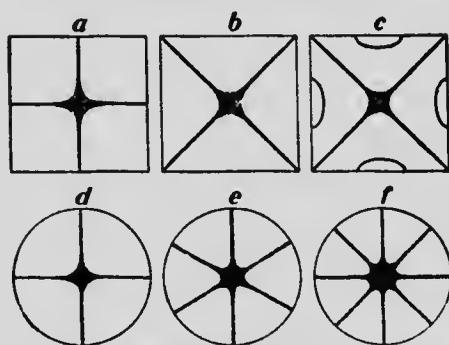
FIG. 221.—Sand-figures showing nodal lines in vibrating plates.
