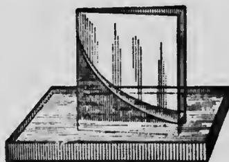
FIG. 183.—Water risen between the two plates of glass which touch along one edge.
