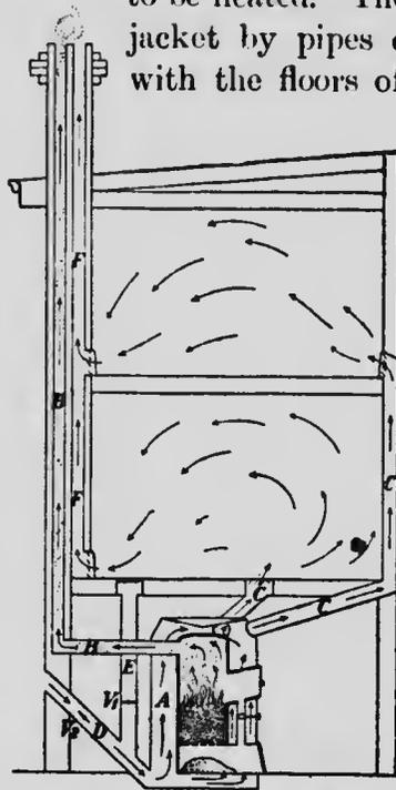
FIG. 317.—Hot air heating and ventilating system. *A*, stove-jacket; *B*, smoke flue; *C*, warm-air pipes; *D*, cold-air pipe from outside; *E*, cold-air pipe from room; *F*, vent flue; *V*<sub>1</sub>, valve in pipe *E*; *V*<sub>2</sub>, valve in pipe from outside.
