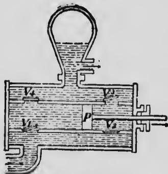
Fig. 159. — Double-action force-pump.
