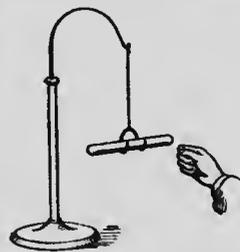
FIG. 461.—The electrified rod moves towards the hand.
