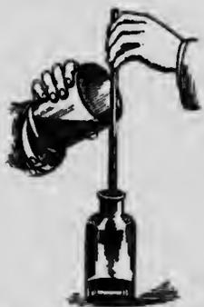
Fig. 185.—How to utilize surface tension in pouring a liquid.
