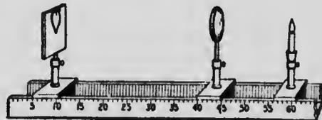
FIG. 396.—An optical bench, for studying object and image.
