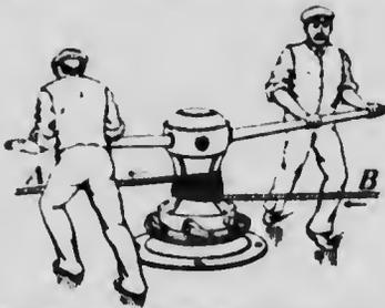
FIG. 90.—Raising the ship's anchor by a capstan.
