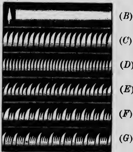
FIG. 236.—Flame pictures seen in the rotating mirror. *A*, when mirror is at rest; *B*, when flame is at rest and mirror rotating; *C*, when a tuning-fork is held before the mouthpiece; *D*, same as *C* but an octave higher; *E*, when *C* and *D* are combined; *F*, obtained with vowel *e* at pitch *C*; *G*, with vowel *o* at the same pitch.
