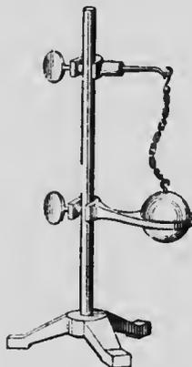
FIG. 254.—Expansion of ball by heat.
