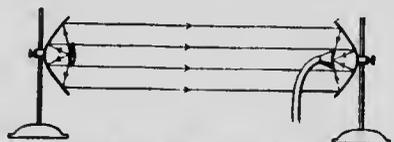
FIG. 208.—A watch is held in the focus of one concave reflector and the ticking is heard at the focus of the other. (The foci can be located by means of rays of light.)
