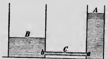
FIG. 473.—Water flows from the higher level in *A* to the lower level in *B*.
