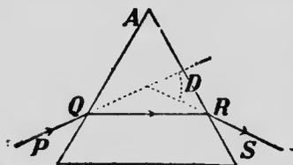
FIG. 376.—The path of light through a prism.
