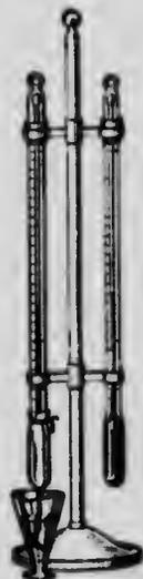
FIG. 290. — Wet-and-dry bulb hygrometer.
