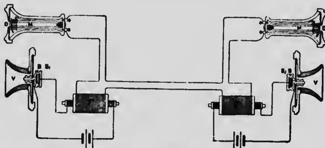
FIG. 552.—Electrical connections in telephone circuit.  $V$ , mouthpiece of transmitter;  $B$ ,  $B_1$ , carbon buttons;  $D$ , diaphragm of receiver, and  $M$  its permanent bar-magnet.  $T$  is a transformer.
