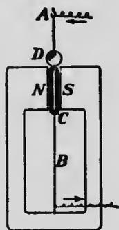
FIG. 523. — The essential parts of a *D'Arsonval galvanometer*.
