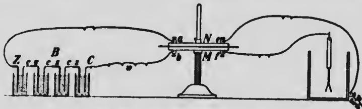
FIG. 486.—The condensing electroscope.
