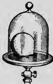
FIG. 139.—Expansion of air when pressure is removed.
