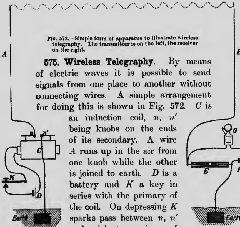
FIG. 572.—Simple form of apparatus to illustrate wireless telegraphy. The transmitter is on the left, the receiver on the right.
