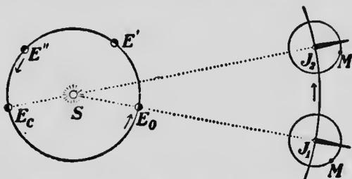
FIG. 331.—Illustrating the eclipse of Jupiter's satellite.  $S$  is the sun,  $E$  the earth,  $J$  Jupiter, and  $M$  its satellite. When the satellite passes into the shadow cast by  $J$  it cannot be seen from  $E$ .
