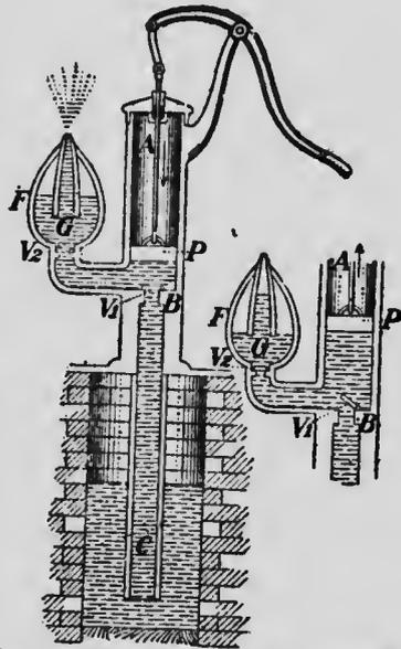
FIG. 158.—Force-pump.  $AB$ , cylindrical barrel;  $BC$ , suction-pipe;  $P$ , piston;  $F$ , air chamber;  $V_1$ , valve in suction-pipe;  $V_2$ , valve in outlet pipe;  $G$ , discharge pipe;  $R$ , reservoir from which water is taken.
