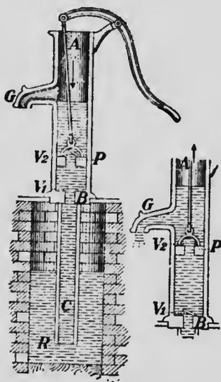
FIG. 157.—Suction-pump. *AB*, cylindrical barrel; *BC*, suction-pipe; *P*, piston; *V*<sub>1</sub> and *V*<sub>2</sub>, valves opening upwards; *R*, reservoir from which water is to be lifted.
