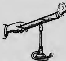
FIG. 302.—Water is a poor conductor of heat.
