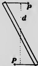
FIG. 41.—Two equal opposite parallel forces produce only rotation.
