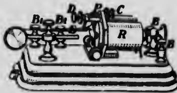
FIG. 519.—Telegraph relay.
