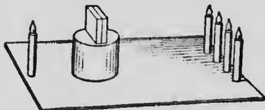
FIG. 329.—If the blocks are equally illuminated the 4 candles are twice as far from the photometer as the single candle.
