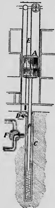
FIG. 108.—Hydraulic elevator.
