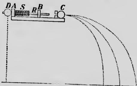
FIG. 33.—The ball *C*, following a curved path reaches the floor at the same time as *D* which falls vertically.
