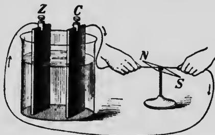
FIG. 487.—Oersted's experiment.
