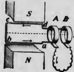
FIG. 533.—Principle of the dynamo.
