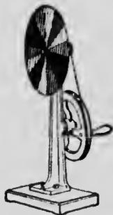
FIG. 406.—Newton's disc on a rotating machine.
