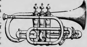
divided into differ- Fig. 249.-By the values a, b, c, the air column is divided into different lengths, and a
