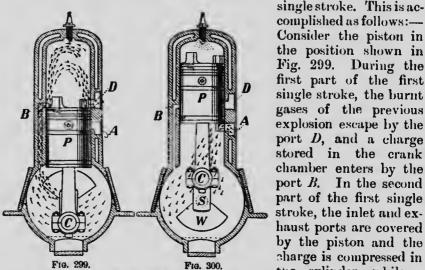
the cylinder, while a Working parts of a two-stroke gas engine. P, piston; S, main shaft; C, crank pin;  $\Delta$ , inlet port to crank char ber; new charge is drawn B, inlet port to cylinder; D, exhaust port; W, counter, 1018 into the crank chamber
