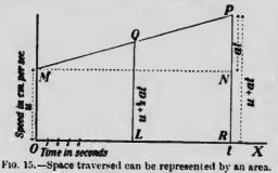
Let distance from Oalong the horizontal line OX represent time in seconds, OR representing tseconds, OL one half of this or  $\frac{1}{2}t$  seconds. Vertical lines represent velocities. The velocity at the beginning u, is represented by OM; that at the end of t se-
