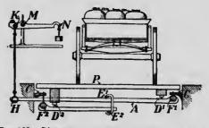
F10. 102.—Diagram of multiplying levers in a scale for weighing hay, coal and other heavy loads. In the figure is shown one half of the system of levers, as seen from one end. The platform Prests on knife-edges  $D^1$ ,  $D^2$ , the former of which is on a long lever, the latter on a short one. The knife-edges  $P^1$ ,  $F^2$  at the ends of these levers are supported by suspension from the brackets C, Cwhich are rigidly connected with the earth.
