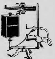
mirror. A section of the gas chamber is shown separately above. On speak-ing into the funnei the flame dances rapidly up and down, and this motion is observed in the square mirror which is rotated by hand.
