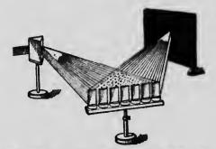
Fig. 405.—The light after passing through the prism falls on several small mirrors which reflect it to one place on the screen. several small plane mirrors, and then by adjusting these properly the various colours may be reflected to one place on the screen, which then appears white (Fig. 405).
