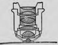
Fig. 412.-A section of an apochromatic microscope objective made by Zeiss.
