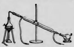
Fig. 291.-Distillation apparatus.
