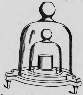
Fig. 6. – United States National Kilogram "No. 20." Kept under two glass bell-jars at Washington. it will not be necessary to use so many decimal places r = 3given here. The equivalent values may be taken from the table opposite page 1.
