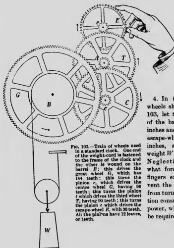
4. In the train of wheels shown in Fig. 103, let the diameter of the barrel B be 2 inches and that of the escape-wheel E be  $1\frac{3}{4}$ inches, and let the weight Whe10 pounds. Neglecting friction, what force must the fingers exert to prevent the escape-wheel from turning? If friction consumes half the power, what force will be required ?
