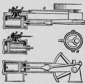
wards by the pressure of steam applied alternately to its two faces (Fig. 294). The steam from the boiler is eouveyed by a pipe F into a valve-chamber, or steam-chest, E. From the steam-chest the steam is admitted to the evlinder by openings ealled ports, A and B, at the ends of the eylinder. The exhanst steam escapes from the cylinder by the same ports. The admission of the steam to the eylinder, and its escape after it has performed its work, is controlled by the op-
