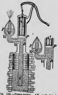
Fig. 158 — Force-pump, AB, cylindrical harrel; BC, suction-pipe; P, piston; F, air chamber;  $V_1$ , valve in suction-pipe;  $V_2$ , valve in outlet pipe; G, discharge pipe; R, reservoir from which water is taken.
