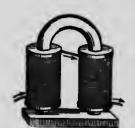
Fig. 510.-An electromagnet-horse-shoe form.
