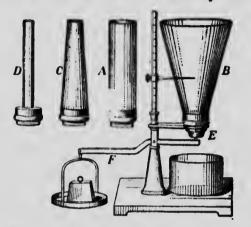
Fig. 113.—Pressures on the bottoms of vessels of different shapes and capacitles.
