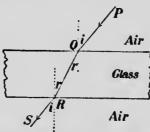
normals at Q and R are parallel, the angles made with these by QR are Fig. 368.—Showing the course of a ray of light through a glass plate.
