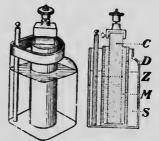
Fig. 489.—Lecianché celi. C. carbon; D. porous cup; Z. zinc; M. carbon and powdered manganese; S. solution of ammonic chloride.
