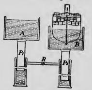
Fig. 110.-Principle of the lift-lock.
