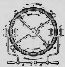
in which, for greater clearness, the two rotating discs are represented as though they were two cylinders of glass, one inside the other and rotating in opposite directions as shown by the arrows.\* The neutralizing brushes  $n_1$ ,  $n_2$  touch the sectors on the back plate, while  $n_3$ ,  $n_4$ touch the front sectors. In the diagram a section of the cylinders is supposed to be seen, and the metal sectors are represented by the dark heavy lines on the outer and inner surfaces.
