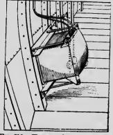
forepeak of the ship, one on each side. The tank is filled with sait water, and the ship's outer skin forms one of its sides. In the water are two microphones, which are connected by wires A, A to two telephone receivers up in the pllot-
