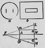
of finding the focal length of a convex mirror.
