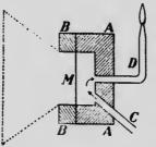
FIG. 237.—A simple form of manometric flame capsule. AA is a cork holiowed out, M is the thin membrane. dotted line, will increase the effect. In place of the rotating mirror a piece of
