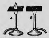
FIG. 304. - Action of metallio gauze on a gas-flame.
