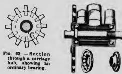
F10 64.— Section of the crank of a bioycle. The cup which holds the balls and the cone on which they on are shown separately elow. Here the balls ouch the cup in two points and the cone in one; it is a "three-point" bearing.
