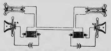
F10. 552.—Electrical connections in telephone circuit.  $V_i$  mouthpiece of transmitter: B,  $B_1$ , carbon buttons; D, diaphragm of receiver, and M its permanent bar-magnet. T is a transformer.
