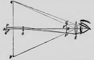
FIG. 403.-Diagram illustrating the compound microscope.
