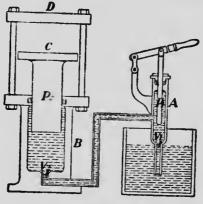
moved by a lever. The bodies to be pressed are held between plates C and D. When  $P_1$  is raised by the lever, water flows up from the cistern through
