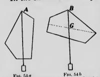
board, let it be supported at A(Fig. 54a) by a pin or in some other convenient way. Have a cord attached to A with a small weight on the end of it.
