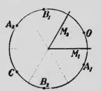
F16. 341. — Images produced by mirrors inclined at an angle of 60°. ference of a circle having the intersection of the mirrors as its centre, and an inspection of the figure will show how to draw them.
