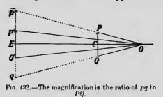
the size of the angle subtended at the eye by the object. Consider the eye to coincide in position with the lens. Then in Fig. 432 the angle subtended at the eye by the object PQ is POQ, that subtended by the image pq is pOq. These angles are identical and at first sight we might think
