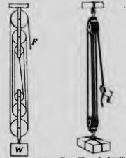
Fig. 83. combination for multiplying the force 6 times.
