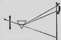
F10, 401.—Light enters through a hole in the window-shutter, passes through a prism and is received on the opposite wall.
