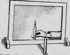
(or other) scale arranged perpendicular to the surface of the glass (Fig. 332). We see an image of the candle on the other side. Now move a second candle behind the glass until it coincides in position with the image.
