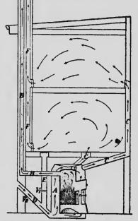
F10. 317.—Hot air heating and ventilating system. A, stove-jacket; B, smoke flue; C, warm air pipes; D, cold-air pipe from outside; E, cold-air pipe from room; F, vent flue; V, valve in pipe E; V<sub>2</sub>, valve in pipe from outside.
