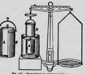
Fig. 121.-Determination of buoyant force.
