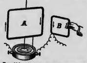
FIG. 512.—Apparatus and connection for demonstrating Ampère's Laws, Paraliel currents in the same direction attract each other.
