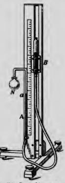
FIG. 273.—Regnault's apparatus for finding the coefficient of expansion of a gas.
