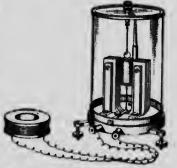
Fig. 527.—Apparatus for showing that when a magnet is thrust into or withdrawn from a closed coil a current is induced in the coil.
