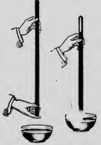
Fig. 127.—Mercury column sustained by the pressure of the air.
