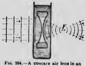
atmosphere of water convergee the light. in water contained in a tank with plate-glass sides.
