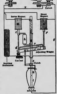
which is at-in the inclosed arc lamp. The iamp iiiustrated in this and the last figure is intended to be joined in series with others on an alternating current circuit, but they are all similar in principle.
