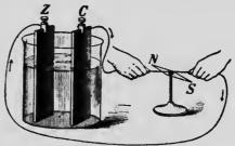
FIG. 487.-Oersted's experiment.
