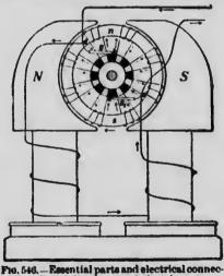
Fig. 546. — Essential parts and electrical connections in the direct-current electric motor. magnetism to cause the machine to develop sufficient current to "pick up" on the start.
