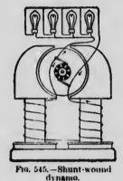
The field-magnets, of course, lose their strength when the current ceases to flow, but the cores contain sufficient residual
