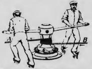
Fig. 90.-Raising the ship's anchor by a capstan.
