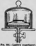
FIG. 284.—Lesile's experiment; freezing water by its own evaporation.
