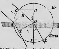
F10. 367.—Diagram to explain the law of refraction. The length of GH is to that of FE as the velocity in air is to that in water.
