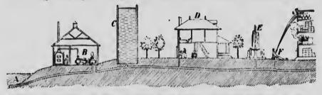
F16, 117.—Water supply system. A, source of water supply; B, pumping station; C, standpipe; D, house supplied with water; E, fountain; F, hydrant for fire hose.
