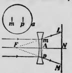
just large enough to cover the lens. Moisten the paper, stick it on the lens, and allow parallel rays to fall on the lens. Now move a screen back and forth until the two bright spots L, M, made by the light passing through the slits, are just twice as far apart as the slits in the paper disc; that is, LM = 2 mp, and LN = 2 mA.
