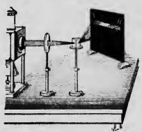
Fig. 402 .- Showing how to produce a pure spectrum.
