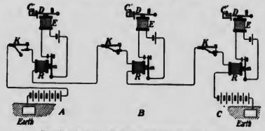
Fig. 520.-Connection of Instruments in a telegraph circuit.
