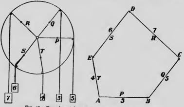
FIG. 45.-Experimental verification of the polygon of forces.
