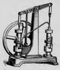
Fig. 148.—An oil air-pump with two cylinders.
