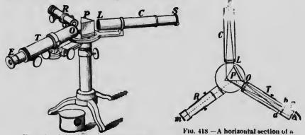
Fig. 417.-A single-prism spectroscope.
