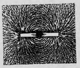
Fig. 451. - Field of lorce ol a bar-magnet.
