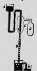
Fig. 150. - Sprengel airpump. A, reservoir into which mercury is poured. B, glass tube of small
