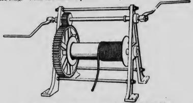
F10. 94 .- Windlam, with gearing, such as is used with a pile-driver.
