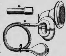
Fig. 247.—Automobile 'honk.' The reed R is shown separately above. It is inserted at r, where the flexible and brass tubes unite.
