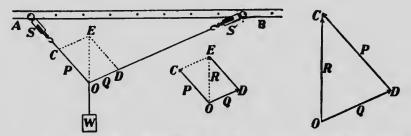
Fig. 43.—How to test the law of parallelogram of forces. Fig. 44.—The triangle of forces.
