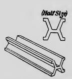
Fig. 2.—View of end and crosssection of the standard 'prototype' metre bars. The line defining the end of the metre is a short mark on the surface midway between the top and bottom of the - s.
