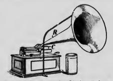
F16. 25). —The phonograph. C is the cylinder on which the spiral groove is made. A cylinder is shown (enlarged) beside the instrument.
