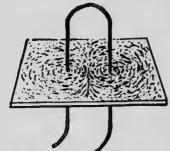
these actions tend to push the wires further apart (see § 499). The directions of the lines of force in the fields may be shown by passing two wires through the card as in the experiment § 498, and causing the current of to pass (1) in the same direction through cach wire (Fig. 515); (2)
