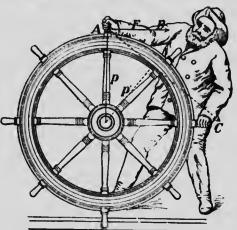
keep the ship on her course the wheelsman grasps the wheel at the rim (i.e., as far as possible from the axis), and exerts a force at right angles to the line joining the axis to the point where he takes hold. (Fig. 36.)
