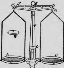
FIG. 8 - A simple and convenient balance. When zero the two masses are equal.
