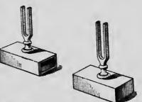
seconds bring it to rest by Fro. 238.-Two tuning-forks arranged to show sympathetic vibrations. When one is vibrated the other responds.
