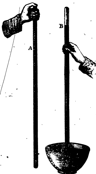
Tube of mercury inverted in a basin of mercury.
