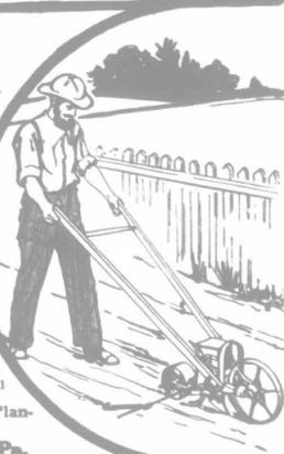
No. 25 Planet Jr. Combined Hill and Drill Seeder, Double Wheel-Hoe Cultivator and Flow opens the furrow, sows the seed accurately in drills or hills, covers, rolls, and marks out next row in one operation. It also has perfect plowing, hoeing, and cultivating attachments.
