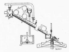
3. In apparatus for effecting separation of minerals by the selective action of oils and like substances, the combination of a conical revolving sieve, a distributor of water shower over part of the sieve, a launder adapted to lead off the matters washed over the sieve, and a launder lined with blanket adapted to lead off the matters that pass through the sieve, substantially as described.
