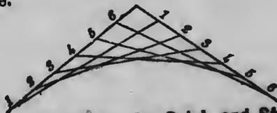
**How to Make the Curves for Brick and Stone Arches.**
