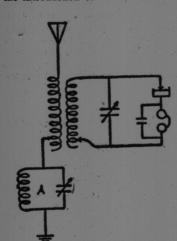
As shown in the accompanying diagram at (A) the absorption of circuit consists of an inductance coil and a variable condenser, so adjusted or tuned to the frequency of the disturbing signal as to reduce the interference after which the receiving circuit is properly tuned to the desired station.
