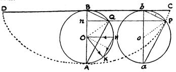
Let the figure represent a common cycloid, traced out by the point P in the circle o whilst the circle rolls along the base C D. The axis is A B and O is the auxiliary circle.
