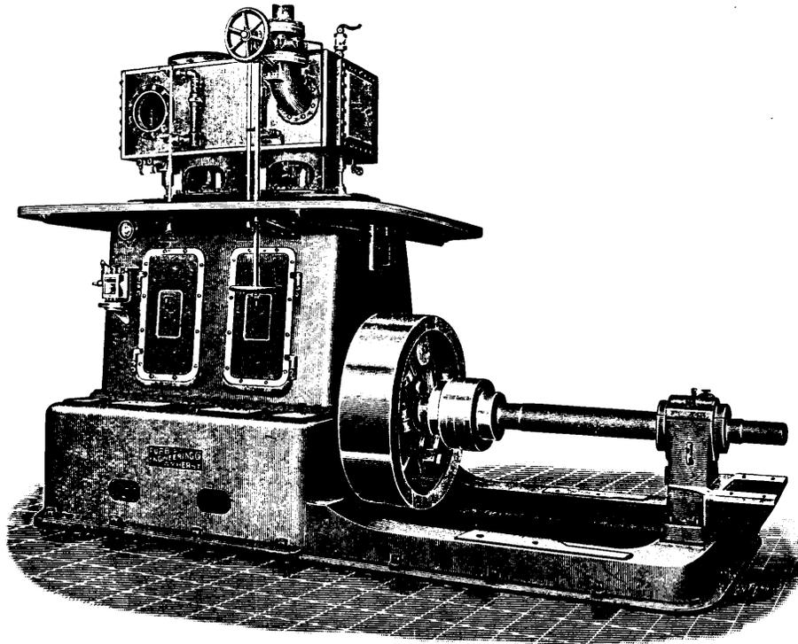
We are prepared to supply High Speed Vertical Enclosed Engines of the English type, up to 750 horse power.
