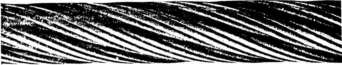
Illustration of Winding Rope, 240 fms. long x 3 1/2 circ. Galvanized Special Improved Patent Steel. Compound Make, supplied to Kenneil Collieries, Bo'ness, Scot., which gave a record life of 6 years and 2 months. Showing condition when taken off.
