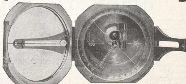
is everywhere recognized as the most convenient, compact and accurate pocket instrument made for preliminary surveying on the surface or underground.
