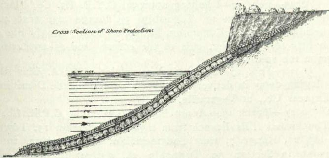
as the mat is in place the river currents produce a scour at the toe of the mat, and unless it is sufficiently flexible to conform to this scour, it is undermined and slips farther into the river, producing a break in the revetment at the water surface.
