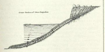
as the mat is in place the river currents produce a scour at the toe of the mat, and unless it is sufficiently flexible to conform to this scour, it is undermined and slips farther into the river, producing a break in the revetment at the water surface.
