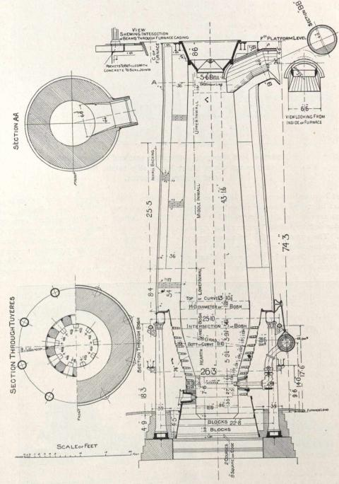
Atikokan Iron Company.-Lines of the Blast Furnace.
