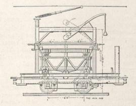
Fig. 6.-Side View of Transfer Car. Showing Lever for Opening
