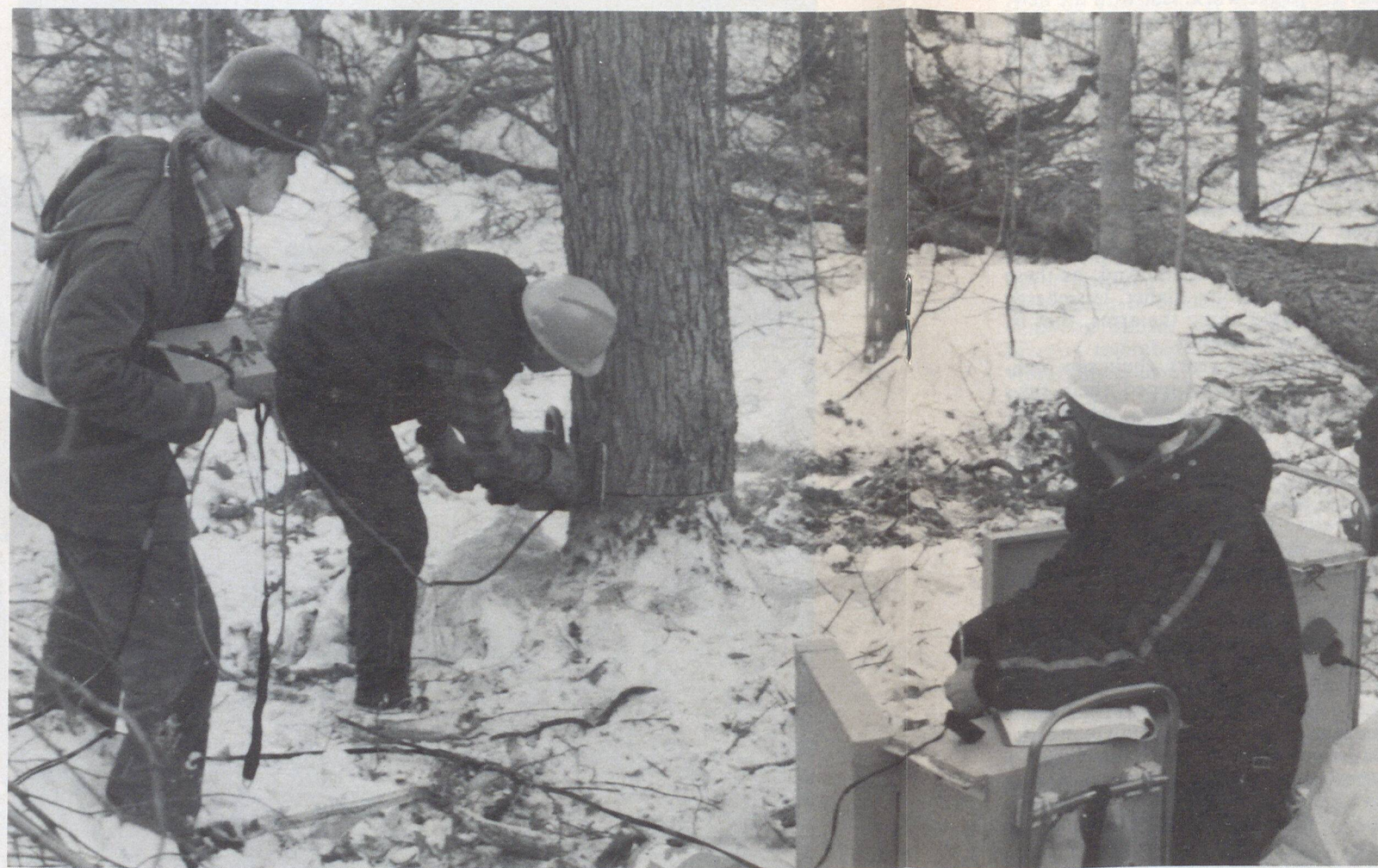
On-site measurement of vibrations during normal chain saw use. A McGill University team combines efforts with NRC's Tony Brammer to help establish safe vibration levels for day-long chain saw use by Canadian operators.
