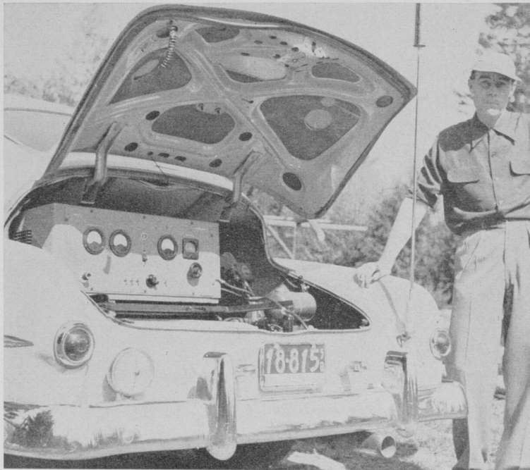
Ranger Jack Betts and radio-equipped automobile. Note steel flanges on which set can be pulled out for inspection.
