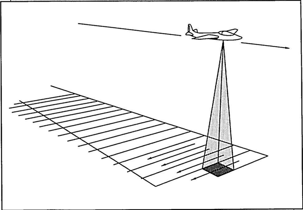
A mirror rotating perpendicular to the line of flight provides the across-track dimension of the imagery. The along-track dimension of the imagery is provided by the motion of the aircraft. (© 1979 by Board of Regents of the University of Wisconsin System. Used with permission.)
