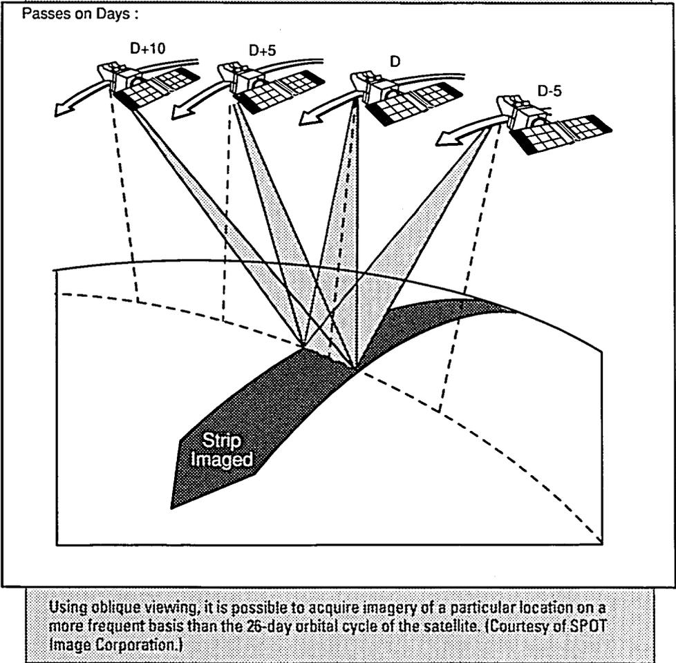
Oblique viewing also reduces the spatial resolution of the images. The raw image line sampling interval (in the across-track direction) at the maximum viewing angle is 13.5 m for panchromatic images and 27 m for multispectral images.<sup>5</sup> In the along-track direction, the column sampling interval remains unaffected by changes in the viewing angle.
