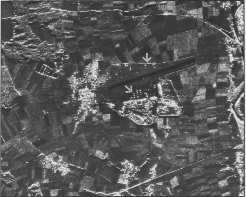
The image was acquired using a SAR with  $3\text{ m} \times 3\text{ m}$  resolution. The aircraft on the tarmac appear as bright returns. The asphalt runway and river are surfaces providing low returns and appear dark. Perimeter fences appear as bright lines, particularly if they are oriented parallel to the aircraft's line of flight when the image was acquired. (Courtesy of Intera Technologies Ltd.)
