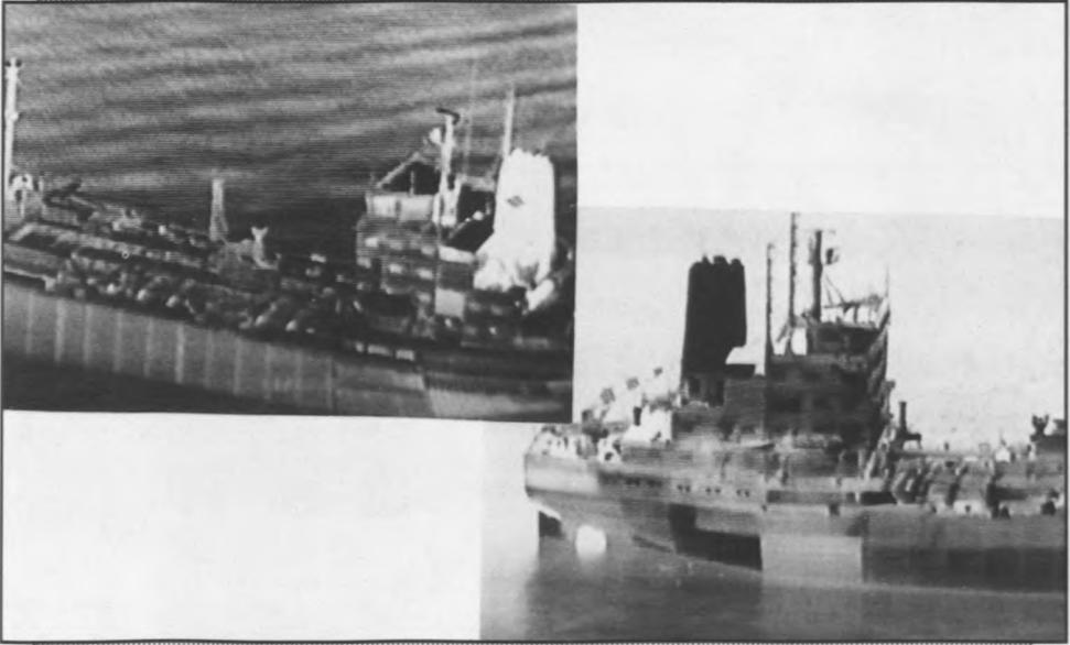
Notice the hot exhaust stack in the left image and the ability to "see through" the hulls of the ships because of the differences in surface temperature resulting from the contents of the holds. (Courtesy of David M. Dorschner, Aviation Resource Management.)
