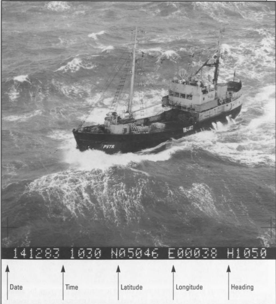
This system has an interface with the aircraft navigation system to annotate basic flight information directly onto the film for each exposure. (Courtesy of Negretti Aviation, Croydon Division.)
