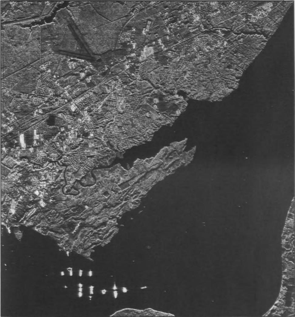
The destroyers seen as bright returns near the bottom of this SAR image are plainly visible but not necessarily easy to identify. Many common cultural features, such as roads, an airport, and housing subdivisions, are evident in the image. (Courtesy of Intera Technologies Ltd.)
