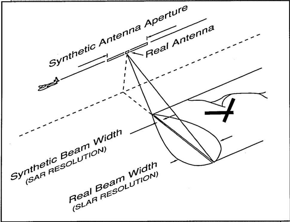
Real aperture radars provide limited spatial resolution because of limitations on the size of antenna that can be mounted onto the aircraft. Synthetic aperture radar systems use the forward motion of the aircraft to create the effect of an antenna hundreds of metres long using a physical antenna size of only one metre. (Courtesy of MacDonald Dettwiler and Associates Ltd.)
