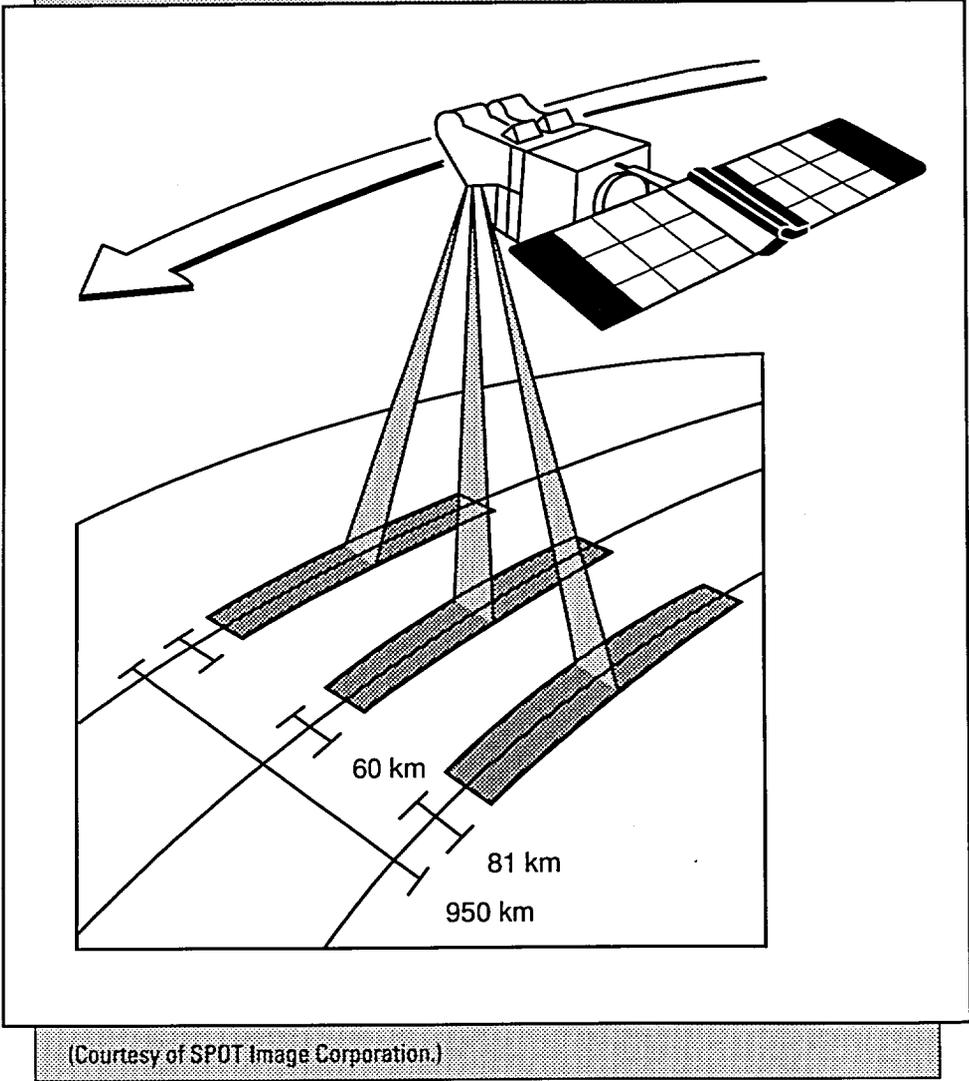
If the satellite were capable of only vertical viewing, it would be possible to image a particular location only once during the 26-day orbital cycle of the satellite. The SPOT satellite's oblique viewing capability provides the means to collect images more frequently for a particular site (Figure 3).<sup>3</sup> At 45° latitude, up to 12 images can be acquired during one 26-day orbital cycle with time intervals from one to four days between successive images.<sup>4</sup>
