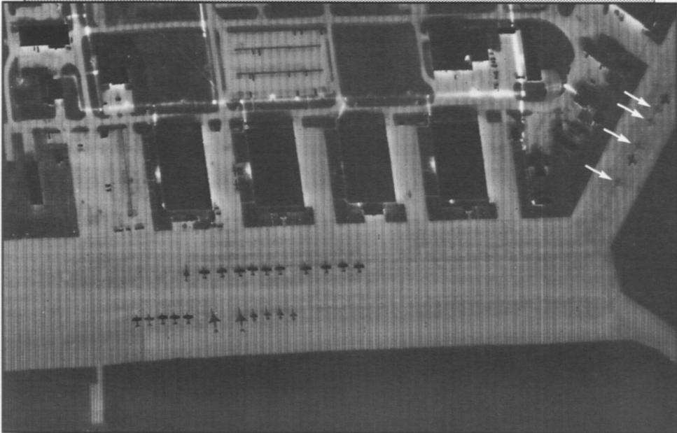
Several types of aircraft can be identified. Thermal shadows remaining in locations where aircraft were parked during the day are also visible (indicated by arrows).
