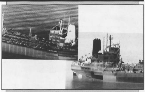
Notice the hot exhaust stack in the left image and the ability to "see through" the hulls of the ships because of the differences in surface temperature resulting from the contents of the holds. (Courtesy of David M. Dorschner, Aviation Resource Management.)
