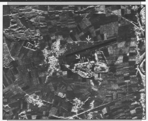
The image was acquired using a SAR with 3 m  $\times$  3 m resolution. The aircraft on the tarmac appear as bright returns. The asphalt runway and river are surfaces providing low returns and appear dark. Perimeter fences appear as bright lines, particularly if they are oriented parallel to the aircraft's line of flight when the image was acquired. (Courtesy of Intera Technologies Ltd.)
