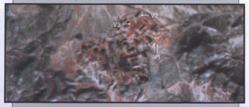
1987/88 change detection overlay image All images © CNES, 1987/88, SPOT Image Distribution. the corresponding 1987 data, the pixel will appear red in the change image. Pixels for which the brightness values have decreased from 1987 to 1988 appear cyan.
