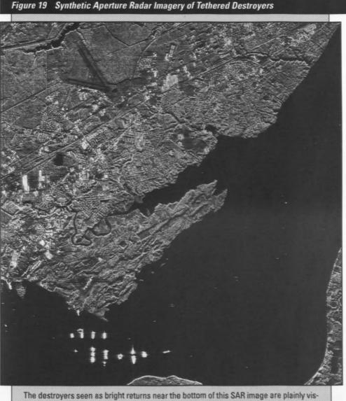
The destroyers seen as bright returns near the bottom of this SAR image are plainly visible but not necessarily easy to identify. Many common cultural features, such as roads, an airport, and housing subdivisions, are evident in the image. (Courtesy of Intera Technologies Ltd.)
