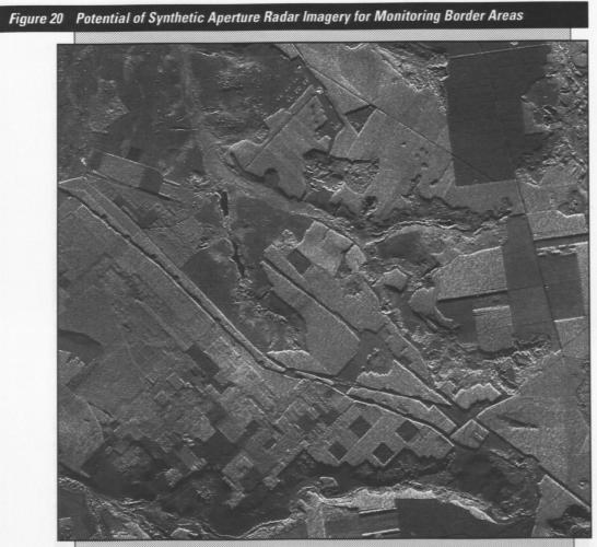
The wide swath coverage and standoff distance provided by SAR imagery could make it useful for this type of monitoring. (Courtesy of Intera Technologies Ltd.)
