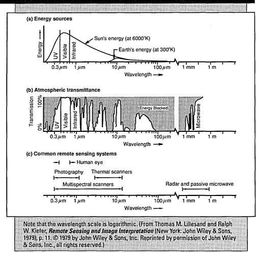
wavelengths and the sensitivity ranges for various sensing systems. The visible light to which our eyes are sensitive includes a small portion, from 0.4  $\mu$ m to about 0.7  $\mu$ m, of the full electromagnetic spectrum.
