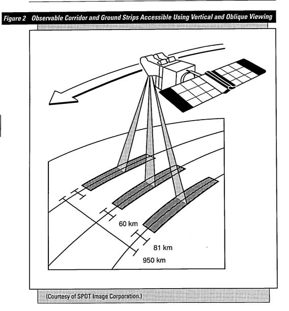
If the satellite were capable of only vertical viewing, it would be possible to image a particular location only once during the 26-day orbital cycle of the satellite. The SPOT satellite's oblique viewing capability provides the means to collect images more frequently for a particular site (Figure 3).<sup>3</sup> At 45° latitude, up to 12 images can be acquired during one 26-day orbital cycle with time intervals from one to four days between successive images.<sup>4</sup>
