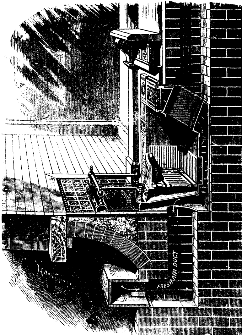
THE JACKSON HEAT-SAVING AND VENTILATING GRATE.
