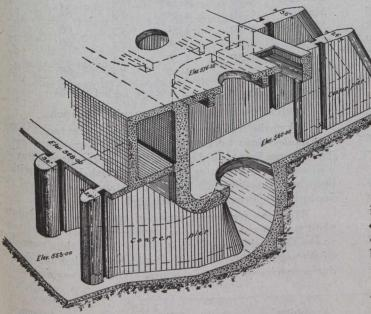
Perspective Sketch Through Substructure Section.
