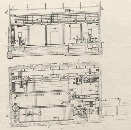
and Monski pump, C<sub>3</sub> and M<sub>3</sub> Jaeger six-stage pump and motor. Measuring channels below the floor are shown. Dimensions are in meters.
