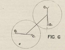
pose the crank pin radius be 12'' and the counterbalance  $O_2$  is set 4" off the centre line; evidently the weight at  $C_1$  acting at 12'' is helped by that at  $O_2$  acting at 4", and the mistake has been made of thinking this weighed the counterbalance at  $O_1$ ; it does not begin to.
