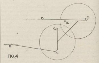
point of view, therefore, the less the overbalance the better, and the problem of the locomotive engineer is to determine to what extent it can possibly be reduced. To discuss this I must refer more in detail to the action of the unbalanced weights on the engine
