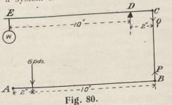
course, there are certain constructional details which cannot be represented in such a figure, but nevertheless this problem illustrates the principle involved in all weighing scales and machines for testing the strength
